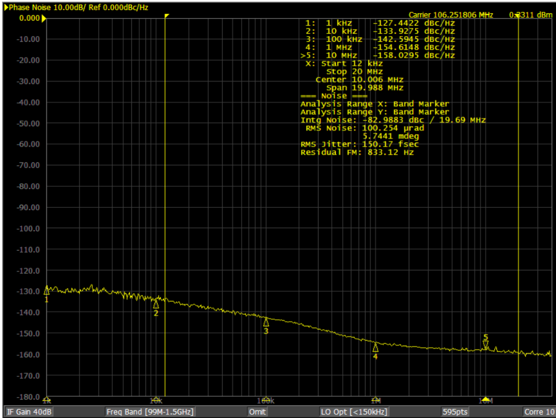
Figure 8. Phase Noise of 106.25MHz Output in Clock Generator Mode
