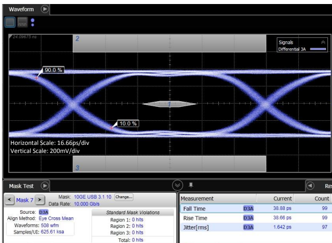
10Gb/s (USB 3.1) Eye Diagram with RClamp3371ZC
