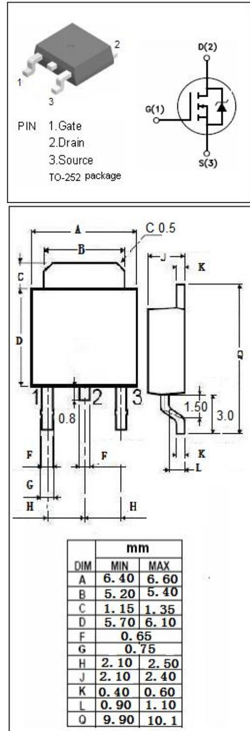
**Isc N-Channel MOSFET Transistor****RD3P050SN****ELECTRICAL CHARACTERISTICS** $T_c=25^\circ\text{C}$  unless otherwise specified
