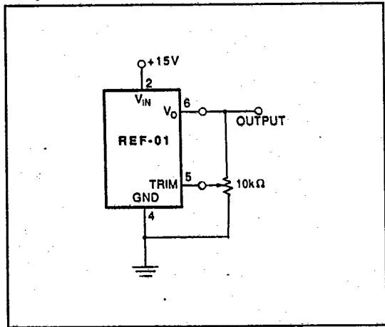
The REF-01 trim terminal can be used to adjust the output voltage over a  $10V \pm 300mV$  range. This feature allows the system designer to trim system errors by setting the reference to a voltage other than 10V. Of course, the output can also be set to exactly 10.000V, or to 10.240V for binary applications.
