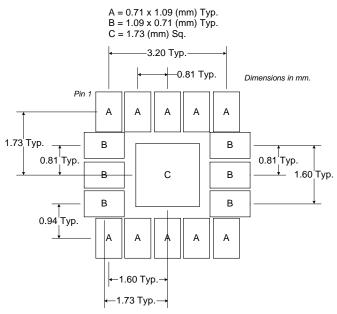
Figure 2. PCB Solder Mask (Top View)
