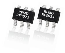
The RF3023 and RF3024 are reflective, single-pole double-throw (SPDT) switches designed for general-purpose switching and battery operated applications which require very low insertion loss and medium power handling capability. Both switches are identical with the exception that their switching logic is reversed. Fabricated with a 0.5µm GaAs pHEMT process, the RF3023 and RF2034 feature low control voltage and moderate isolation. Each comes packaged in a compact SC70, 6-pin package.
