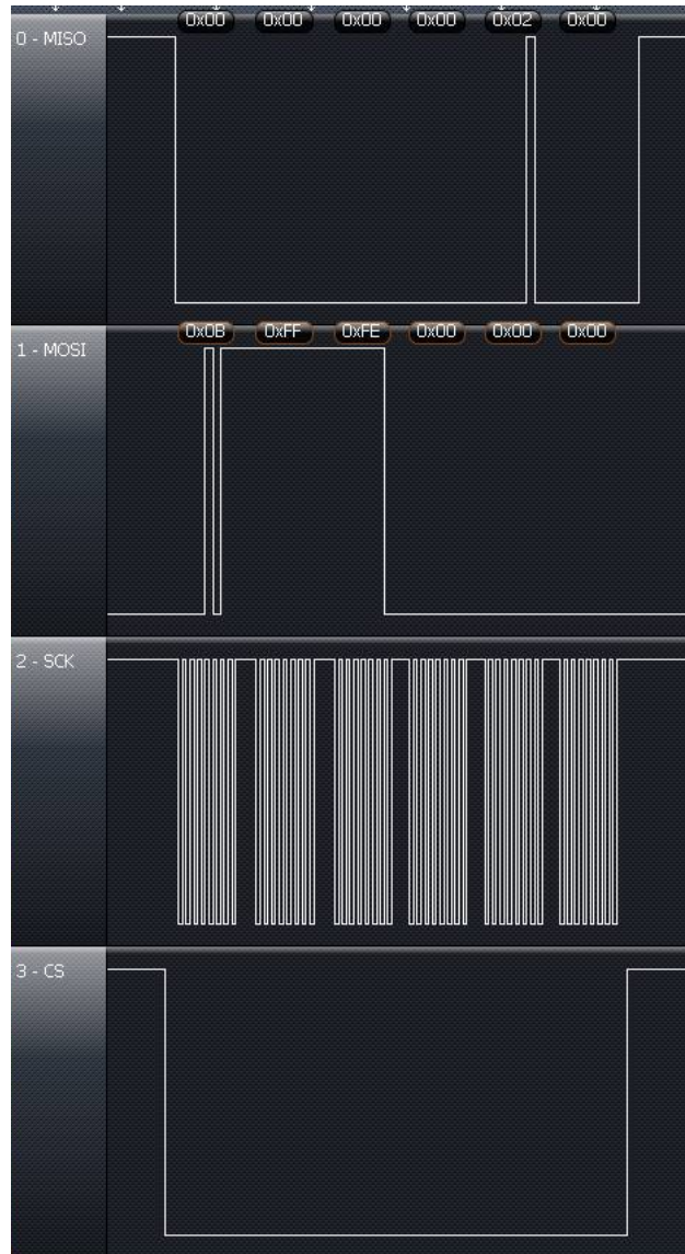
Figure 5-9. SPI Access Example: Read of the Control Register at Address 0xFFFFE, Responds With 0x00, 0x02 (RF Enable = 1)
