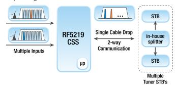
Ground-breaking new technology enables the delivery of up to 4 unique, individually selected channels down to a single cable drop.
