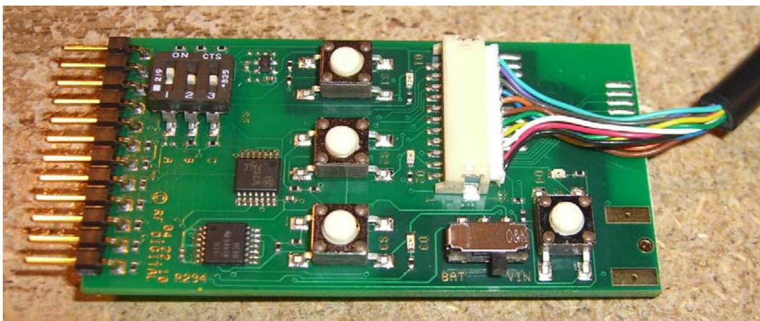
RFD21740 Eval board with RFDANT RFD21743 plugged into the eval board connector. This is a polarized connector and there is only one way to plug in the connector. The black wire is ground and is located close to the slide switch as shown below. The RFD21740 functions exactly like the RFD21737.
