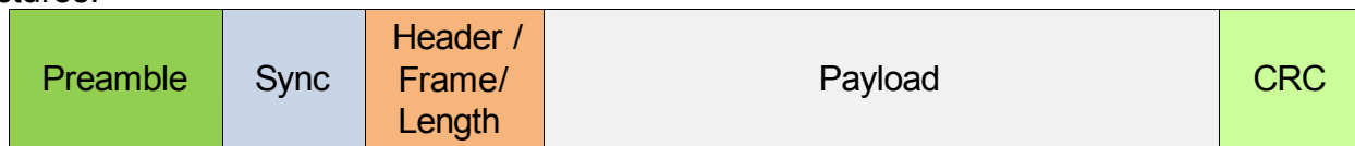
Figure 12. Packet Handler Structure
