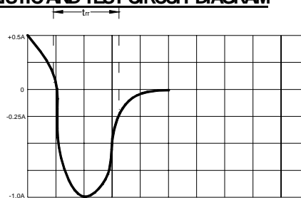
FIG.1 – REVERSE RECOVERY TIME CHARACTERISTIC AND TEST CIRCUIT DIAGRAM
