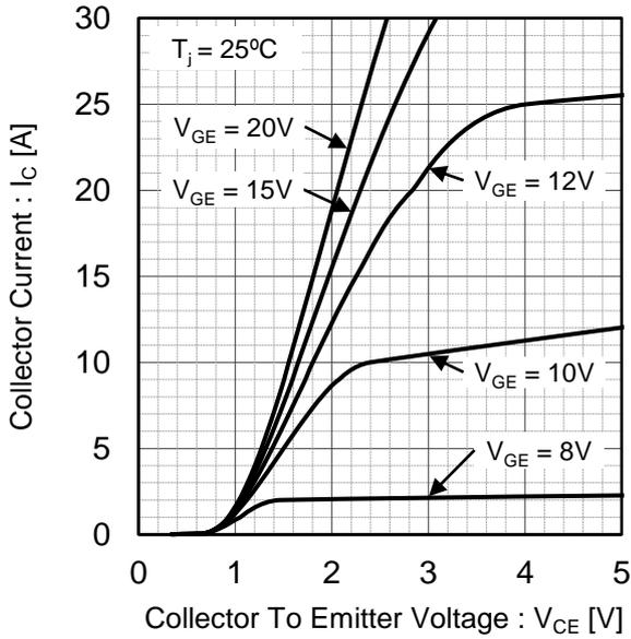
Fig.6 Typical Output Characteristics
