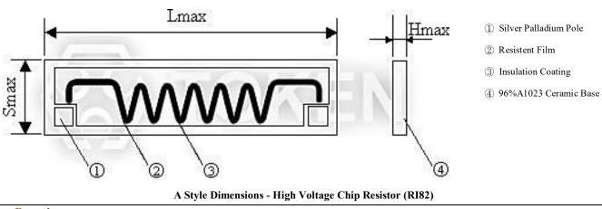
• Remark: Rated continuous Working Voltage (RCWV) shall be determined from RCWV =  $\sqrt{\text{Power Rating} \times \text{Resistance Value}(\Omega)}$ . When RCWV  $\geq$  Max. Working Voltage listed above, RCWV = Max. Working Voltage.
