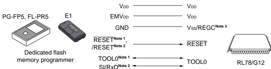
Figure 24-2. Communication with Dedicated Flash Memory Programmer
