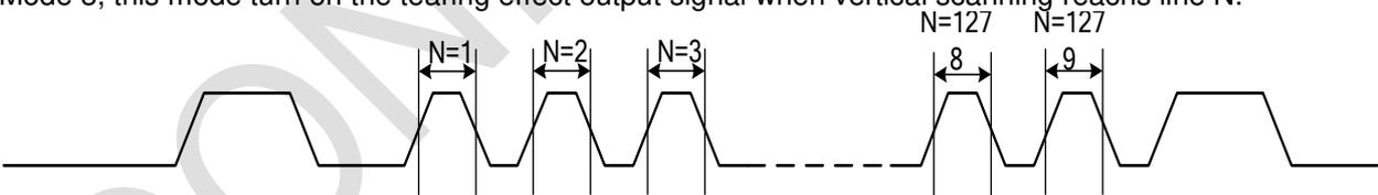
N = The N-th scanning line which set by register N[15:0] of command `STESL`(44h).
