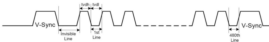
**The Tearing Effect Output line shall be active low when the display module is in Sleep mode.**
