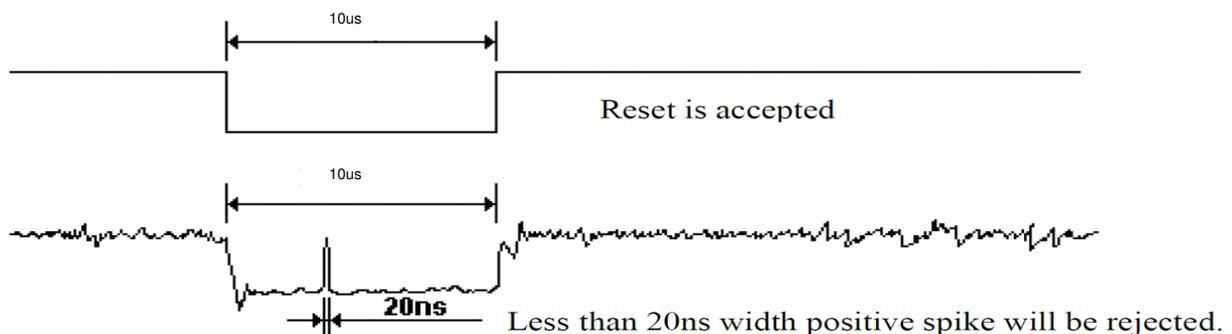
Note 5. It is necessary to wait 5msec after releasing RESX before sending commands. Also Sleep Out command cannot be sent for 120msec.
