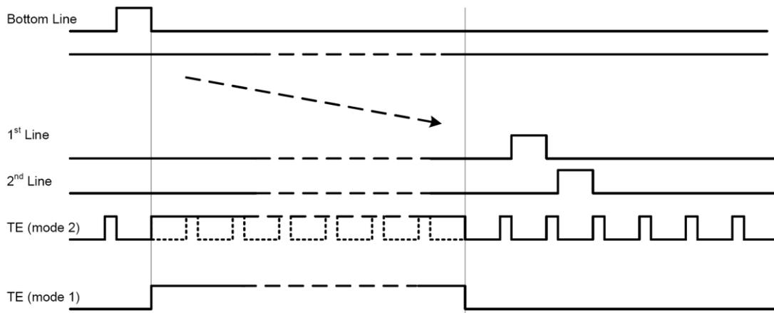
Note. During Sleep In mode, the tearing effect output signal is active low.
