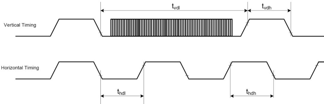
AC characteristics of Tearing Effect Signal (Frame Rate = 60.5Hz)
