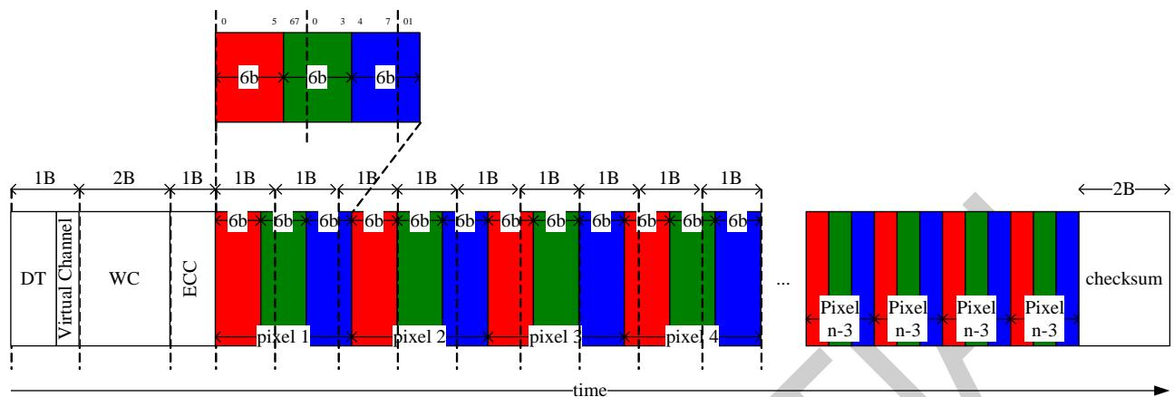
Packet pixel stream, 18-bit format in three bytes, Data Type: 10 1110
