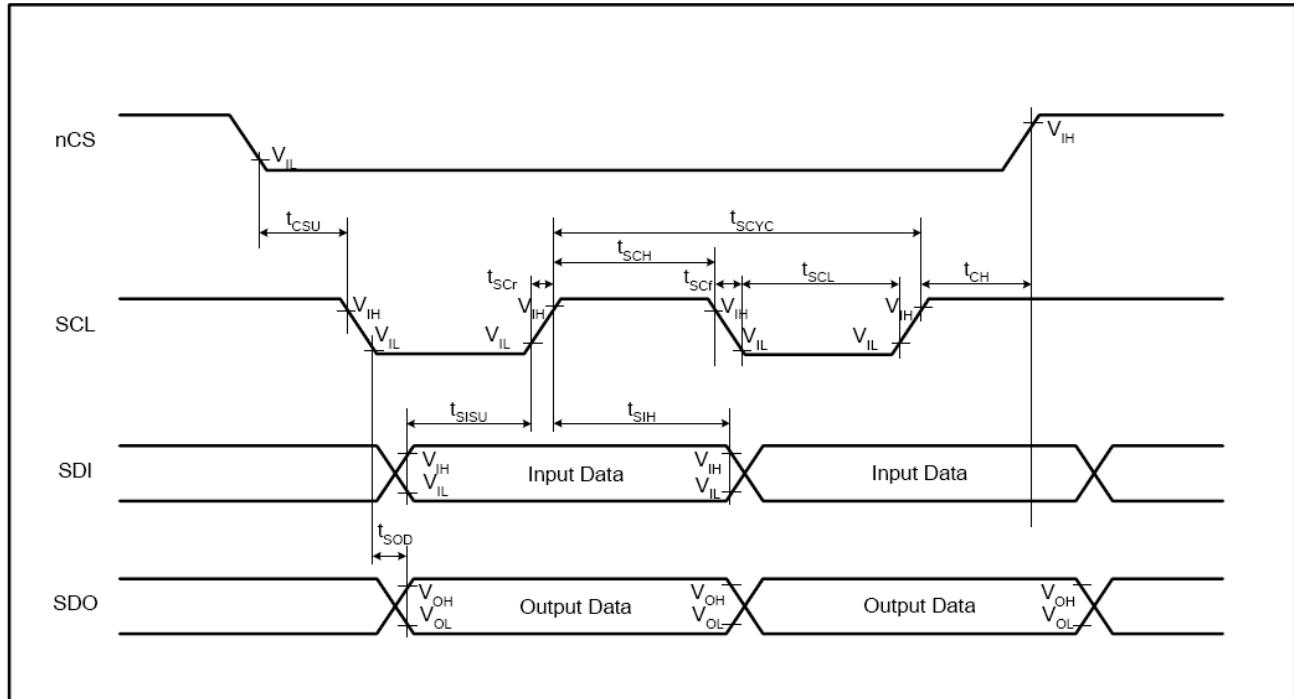
4-Wire SPI Serial Interface Characteristics
