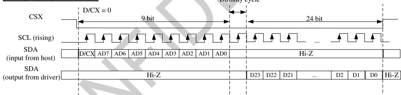
**4-wire SPI (0Ah/0B/0Ch/0Dh/0Eh/0Fh/DAh/DBh/DCh) for 8 bit read**
