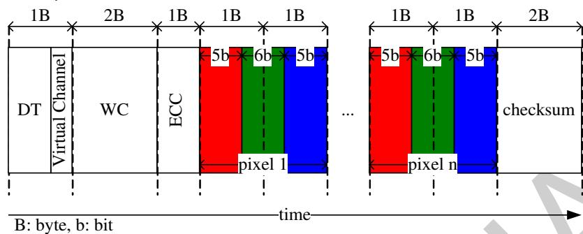
Packet pixel stream, 18-bit format, Data Type: 01 1110
