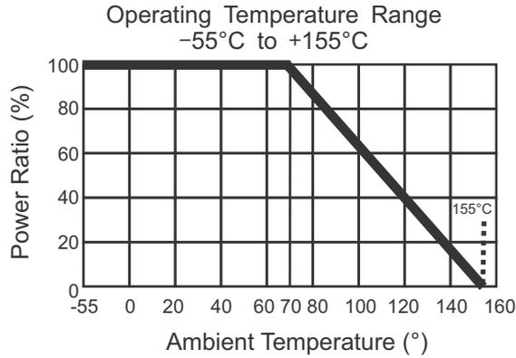
Power rating or current rating is in the case based on continuous full-load at ambient temperature of 70°C. For operation at ambient temperature in excess of 70°C, the load should be derated in accordance with figure of derating Curve.
