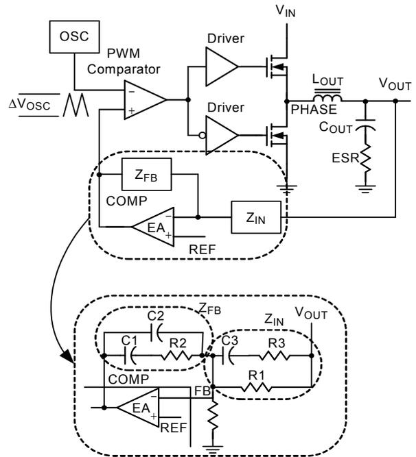
Figure 3. Control Loop for Voltage Mode Buck Converter
