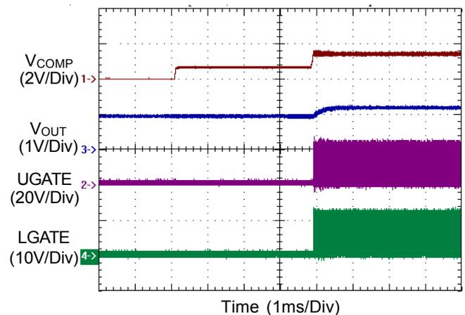
Figure 1. Power Up with Pre-Biased Output Voltage
