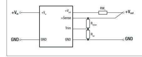
The output voltage can be adjusted via the trim and sense functions.
