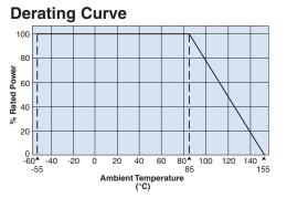
For resistors operated at an ambient temperature of 85°C or above, a power rating shall be derated in accordance with the derating curve.
