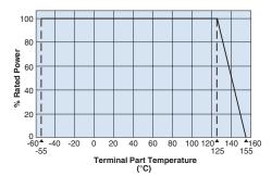
For resistors operated terminal part temperature of described for each size or above, a power rating shall be derated in accordance with the derating curve. Please refer to "Introduction of the derating curve based on the terminal part temperature" in the beginning of our catalog before use.
