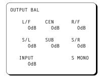
The OUTPUT BALANCE screen provides a temporary adjustment to the relative output levels of each speaker in the system. Unlike the BALANCE CHECK calibration procedure, the changes made on this screen are temporary. They change the output balance only for the current source input and only until a different source is selected, when the settings will revert to the system-wide default established during the BALANCE CHECK calibration.
