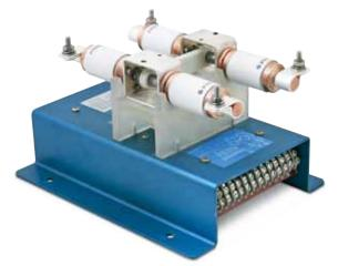
RT22-4070-A31NB and RT22-4070-A317B are vacuum contactors with DPDT contact arrangements. These units can also be used as SPDT contactors by wiring the contacts in parallel. These contactors are commonly used in antenna switching for high power RF circuits, such as those encountered in transmitters.
