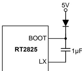
Figure 9. External Bootstrap Diode
