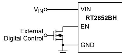
Figure 3. Digital Enable Control
