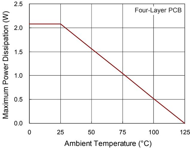
Figure 10. Derating Curve of Maximum Power Dissipation
