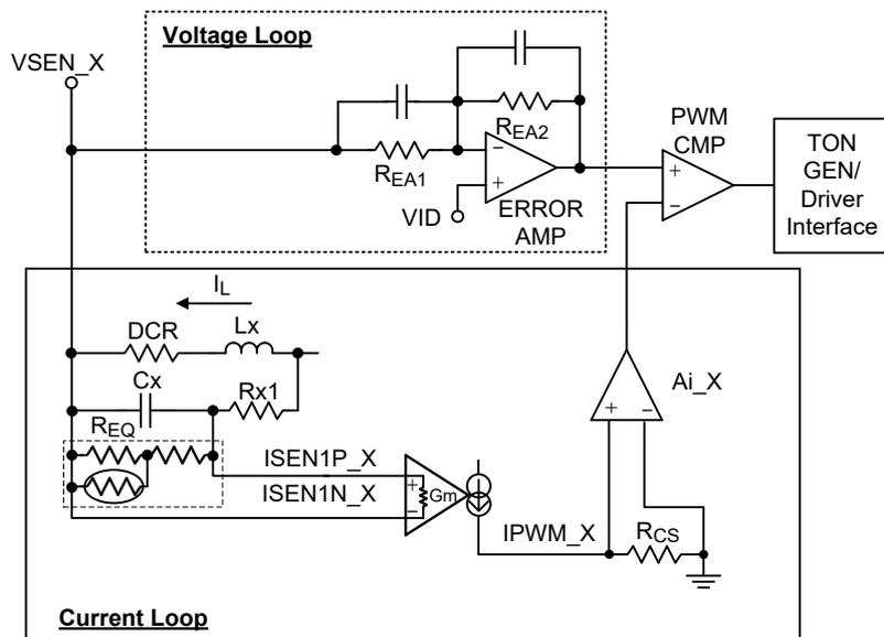
Figure 26. Voltage Loop and Current Loop for Load-line
