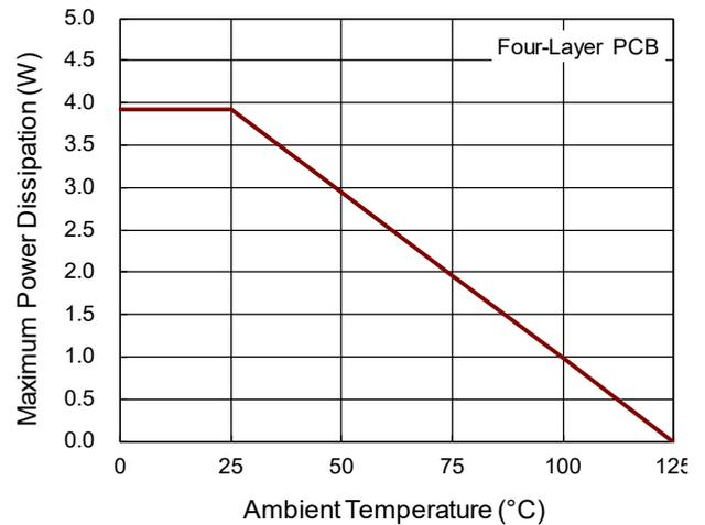
Figure 37. Derating Curve of Maximum Power Dissipation
