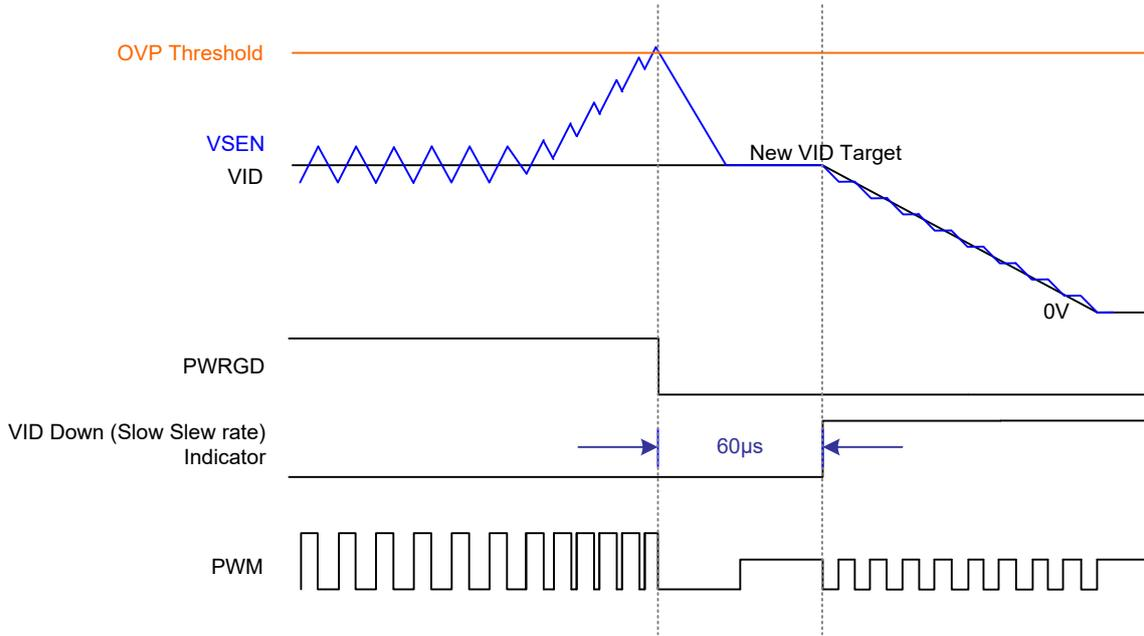
Figure 35. Overvoltage Protection Mechanism
