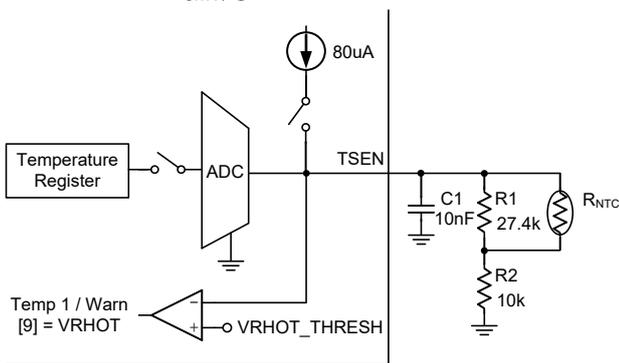
Figure 4. Multi-Function Pin Setting Mechanism for TSEN
