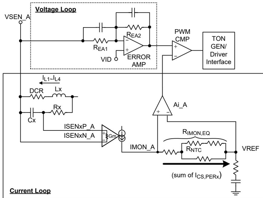
Figure 13. Voltage Loop and Current Loop for Load-line
