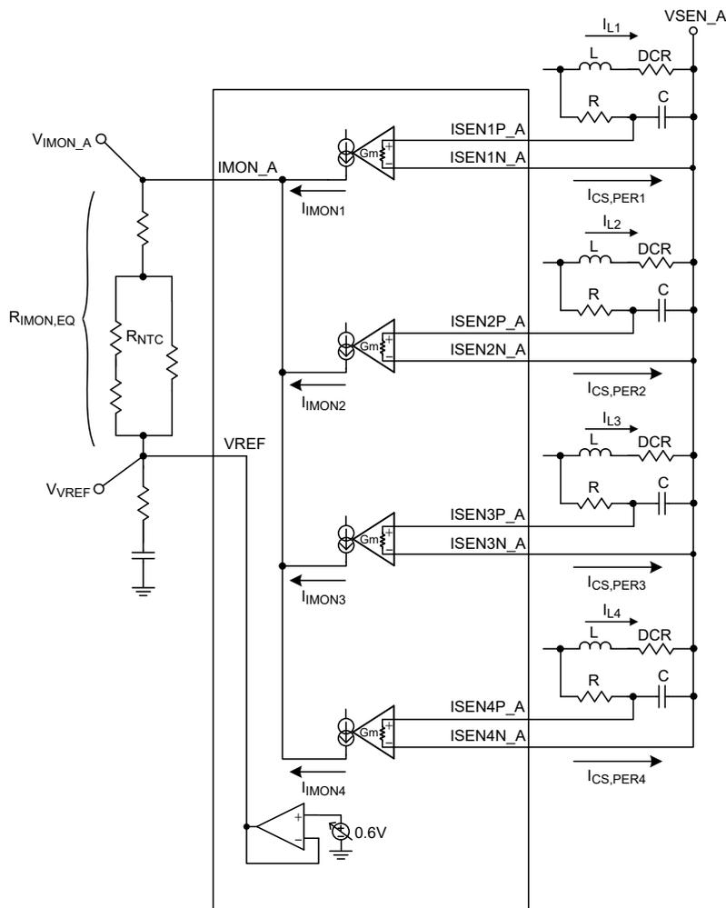
Figure 10. Total DCR Current Sense Method
