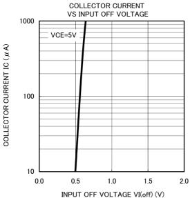
Composite Transistor With Resistor For Switching Application Silicon Epitaxial Type
