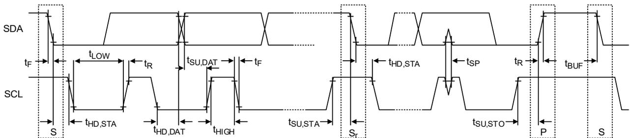
Figure 4. I<sup>2</sup>C Read/Write Stream and Timing Diagram
