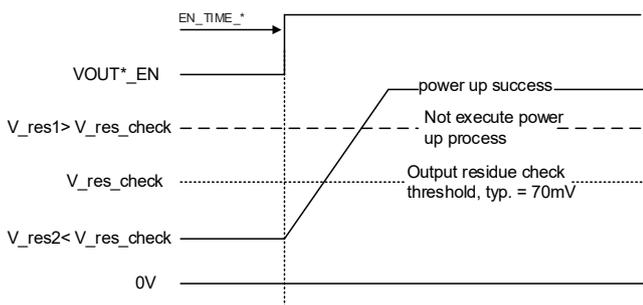
Figure 8. Output Residual Voltage Check During Power-Up Process
