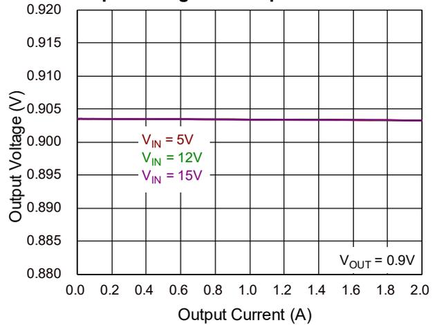
**Buck3 Output Voltage vs. Output Current in FCCM**
