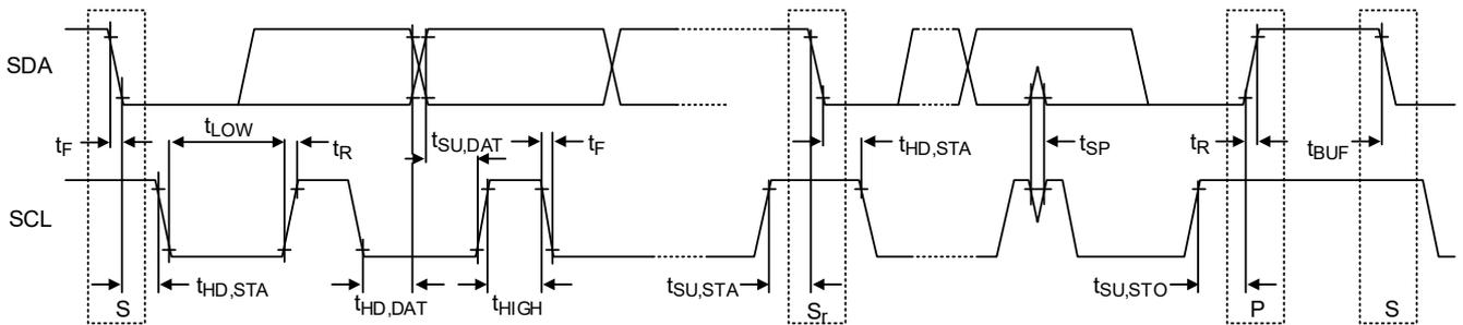
Figure 12. I<sup>2</sup>C Waveform Information
