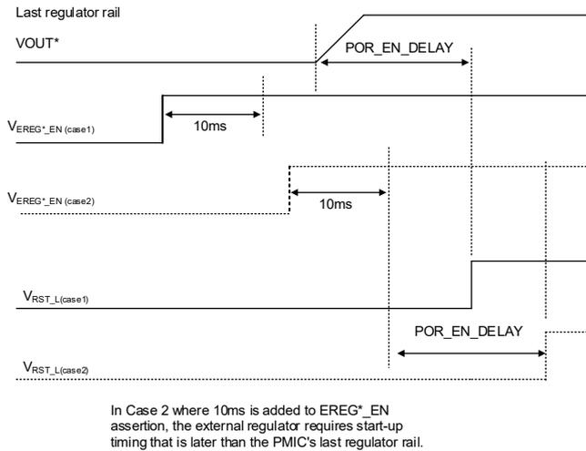
Figure 4. Power-Up Process Completion and RST\_L Assertion
