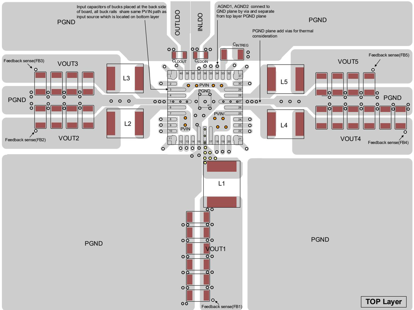
Figure 14. PCB Layout Reference of Option 1 (Top Layer)
