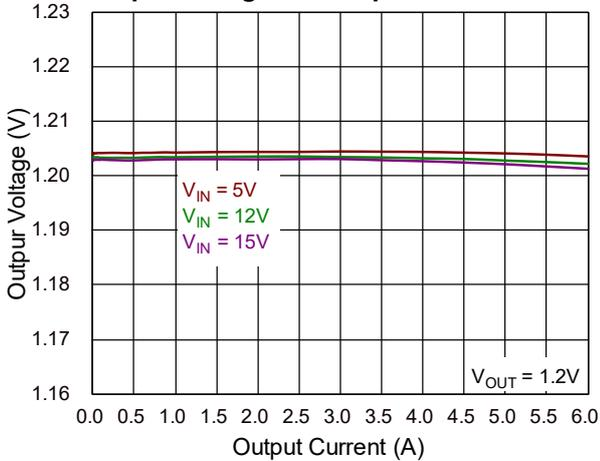
**Buck2 Output Voltage vs. Output Current in FCCM**
