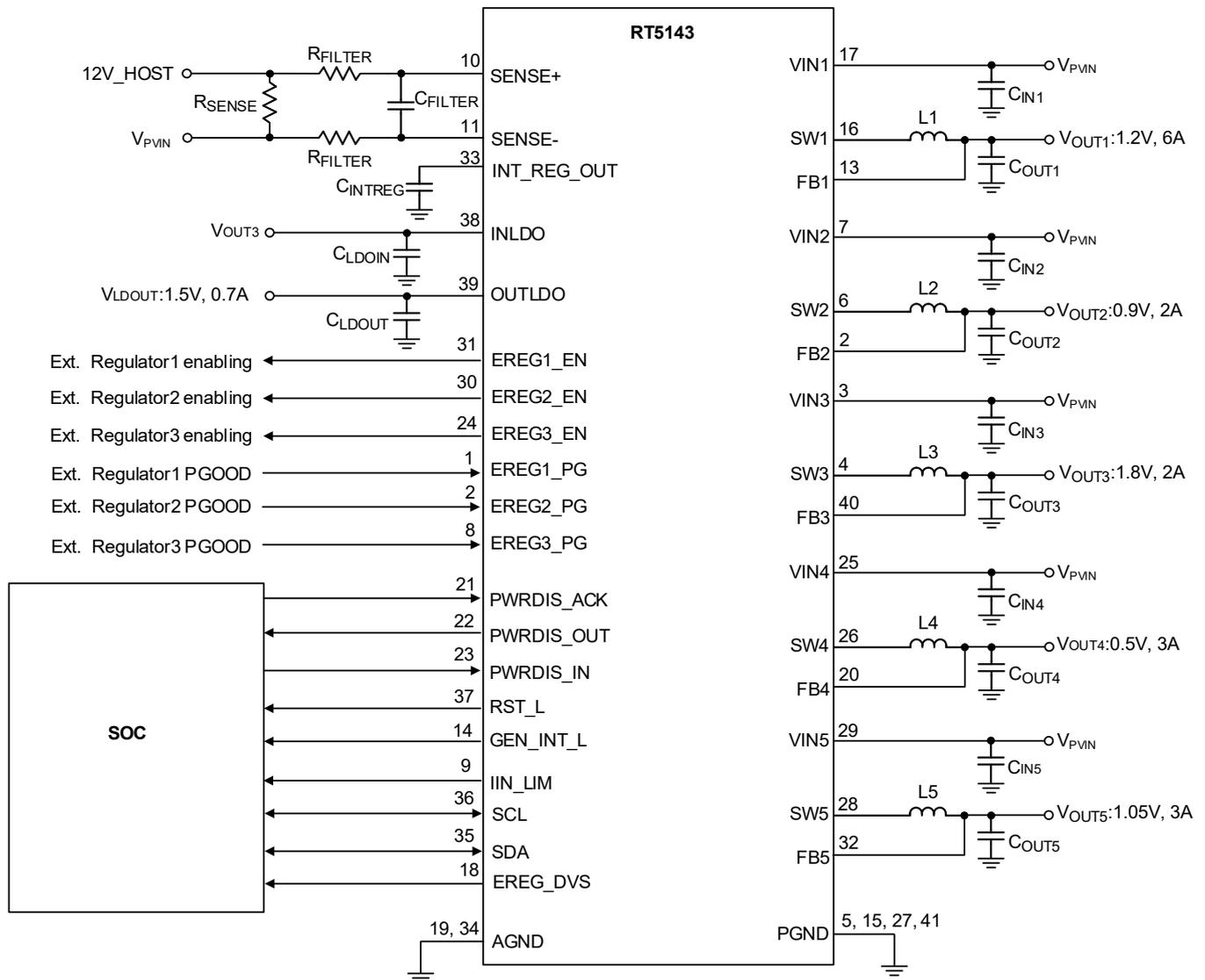
Figure 5. Application Circuit for Buck Normal Mode Operation
