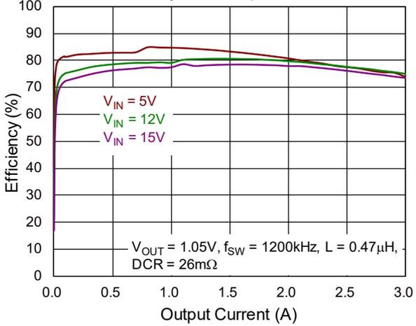
**Buck5 Efficiency vs. Output Current in FCCM**
