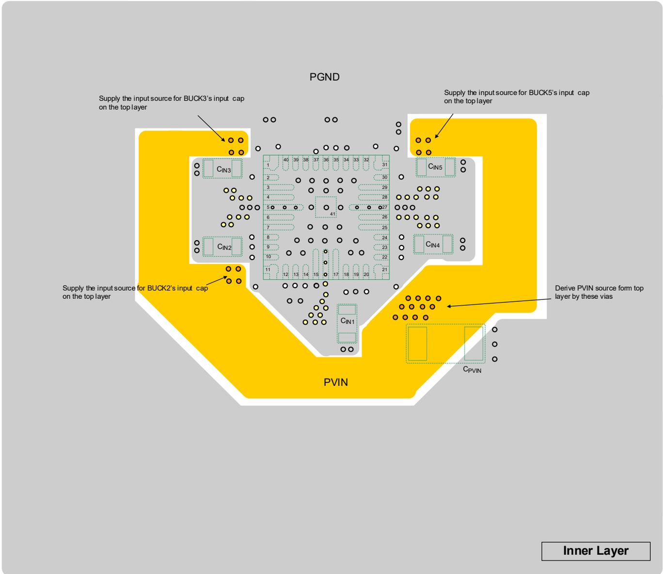
Figure 17. PCB Layout Reference of Option 2 (Inner Layer, top view)
