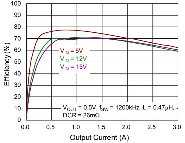
**Buck5 Efficiency vs. Output Current in PSM**
