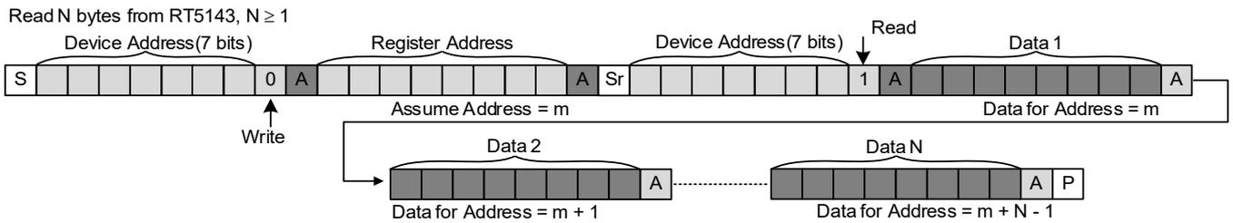
Figure 11. I<sup>2</sup>C Read Access Multiple Bytes
