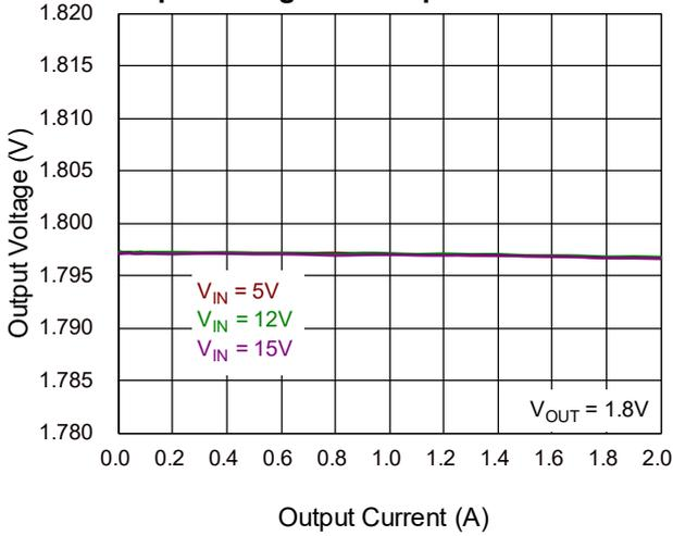
**Buck4 Output Voltage vs. Output Current in FCCM**
