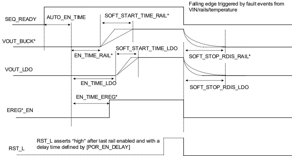
Figure 7. Rail Power-On and Power-Off Procedure
