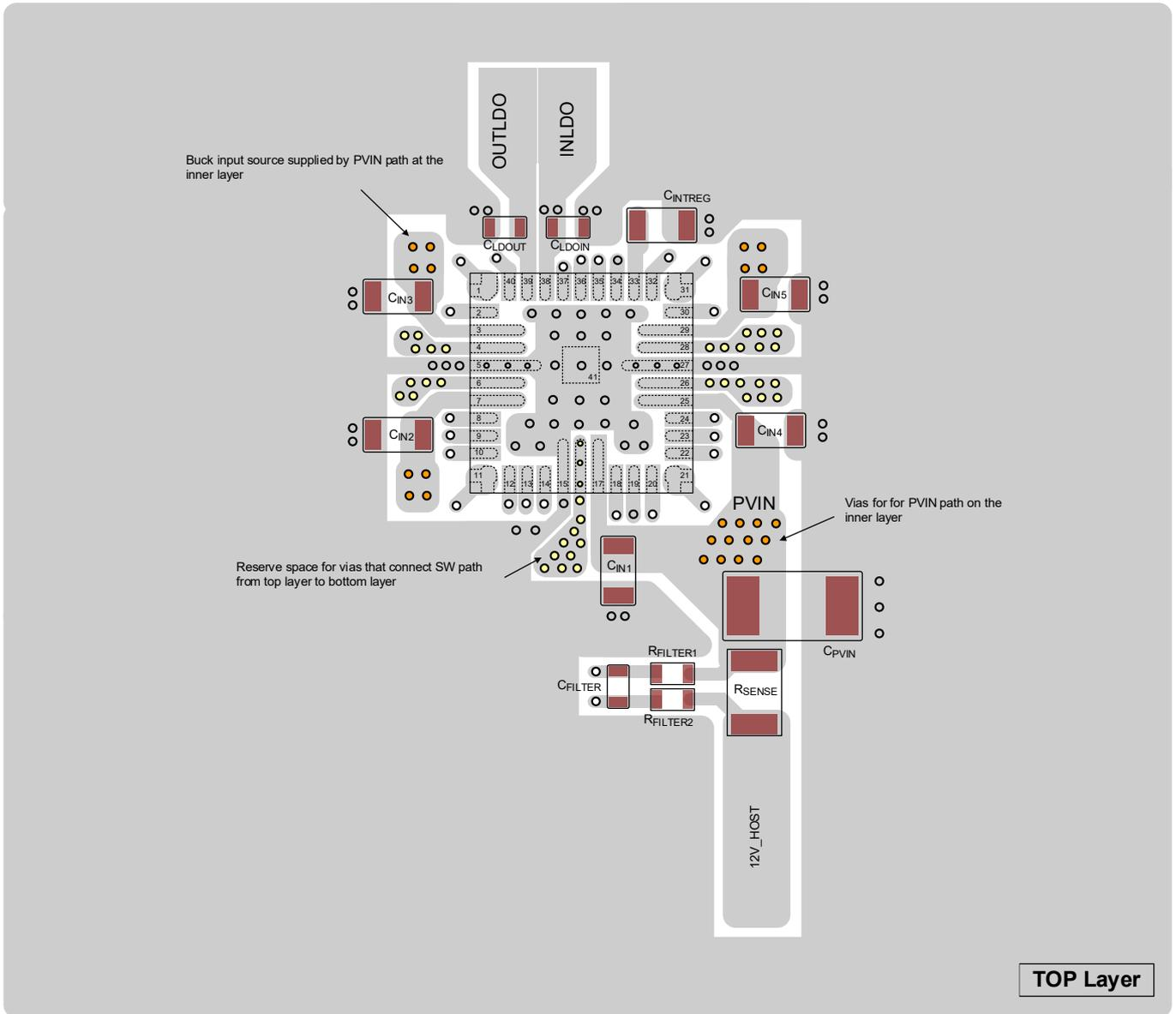
Figure 16. PCB Layout Reference of Option 2 (Top Layer)
