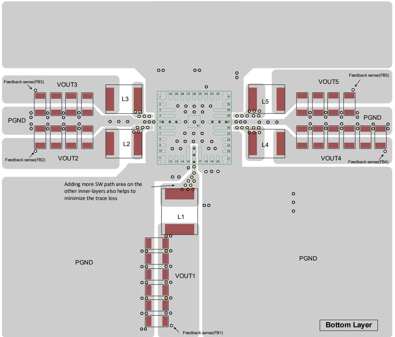
Figure 18. PCB Layout Reference of Option 2 (Bottom Layer, top view)
