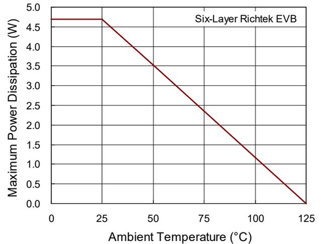
Figure 13. Derating Curve of Maximum Power Dissipation
