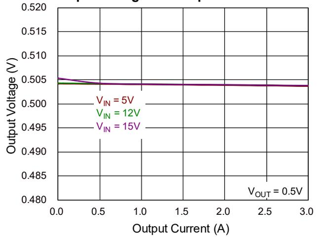
**Buck5 Output Voltage vs. Output Current in FCCM**
