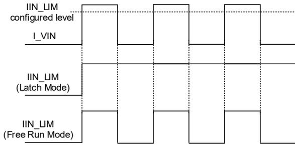
Figure 9. IIN\_LIM “Latch Mode” and “Free Run Mode” Operation
