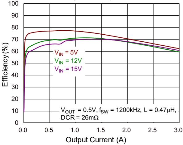
**Buck4 Efficiency vs. Output Current in FCCM**
