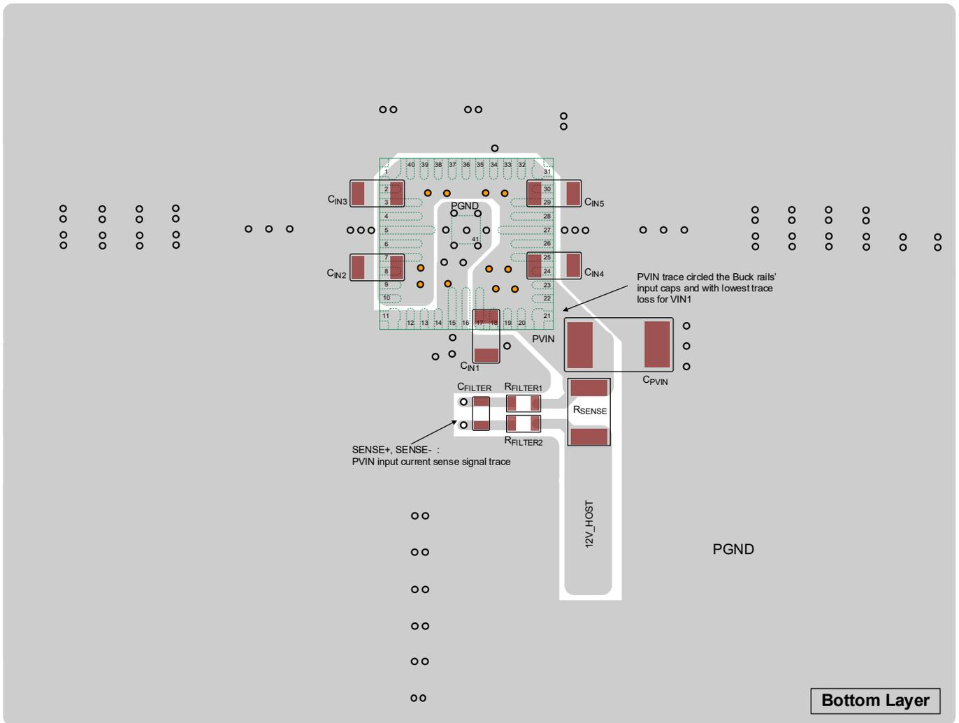
Figure 15. PCB Layout Reference of Option 1 (Bottom Layer, top view)
