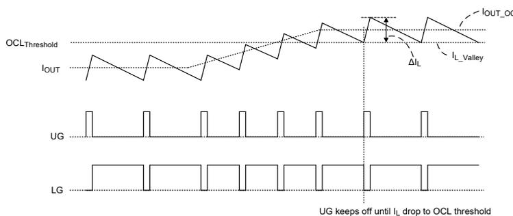
Figure 1. Cycle-by-Cycle “Valley” Current Limiting Control
