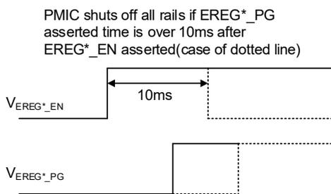
Figure 2. Power-Up Process Interrupted by EREGx\_PG Status
