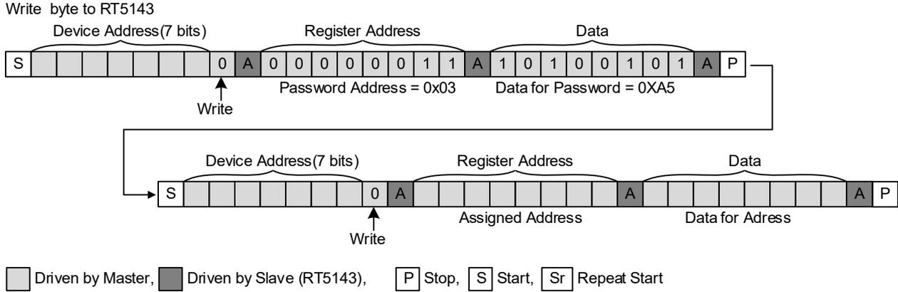
Figure 10. I<sup>2</sup>C Write Access Byte
