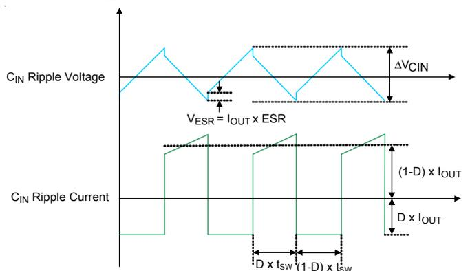
Figure 4. C<sub>IN</sub> Ripple Voltage and Ripple Current
