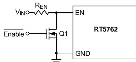
Figure 7. Logic Control for the EN Pin
