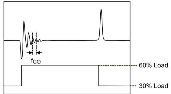
Figure 10. Example of Measuring the Converter f<sub>CO</sub> by Fast Load Transient
