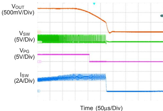
Figure 2. Over-Current Protection
