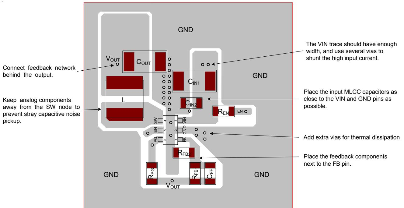
Figure 12. Layout Guide for SOT-563 (FC)
