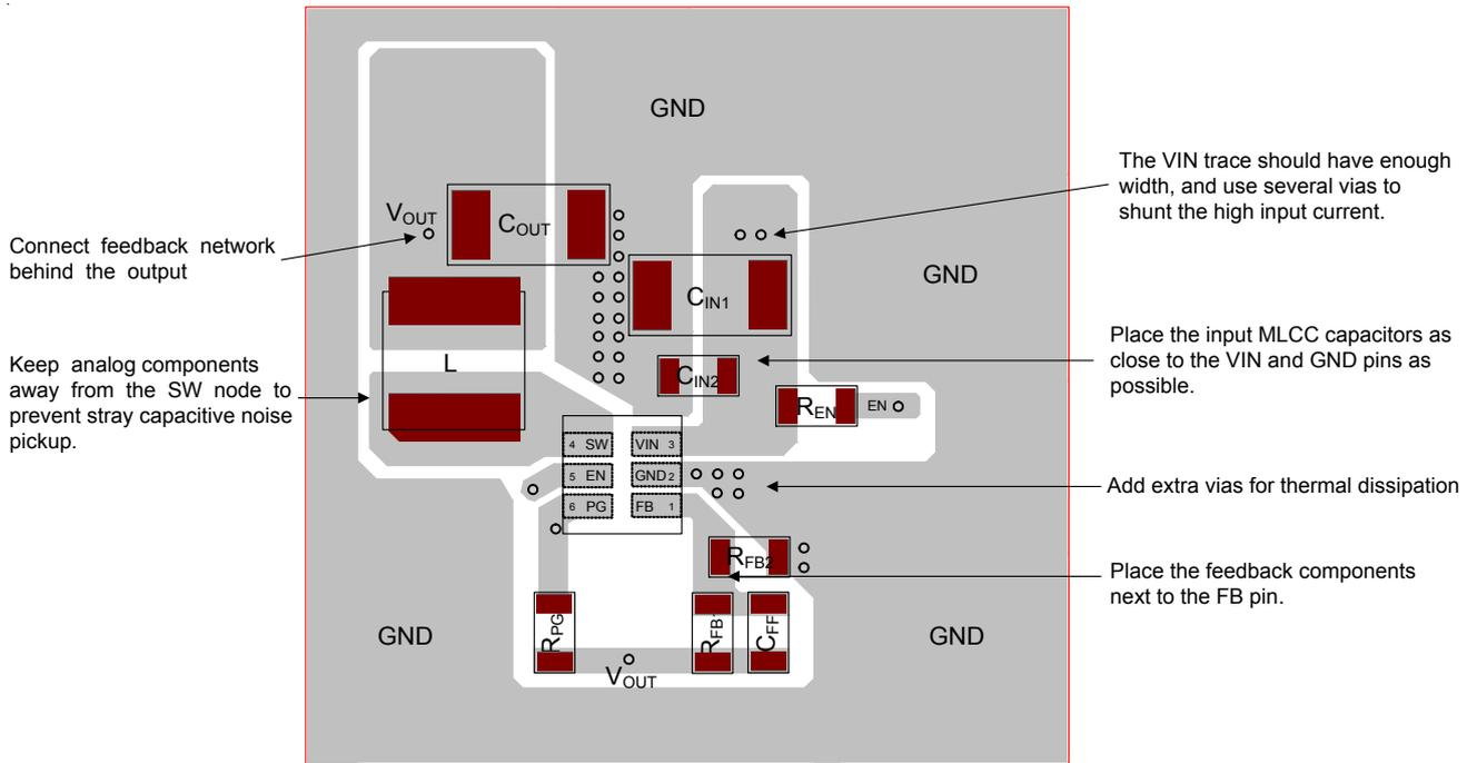
Figure 13. Layout Guide for UDFN-6L 1.4x1 (FC)
