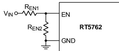
Figure 8. Resistive Divider for Under-Voltage Lockout Threshold Setting
