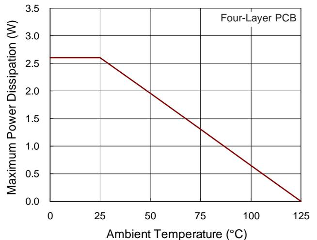
Figure 2. Derating Curve of Maximum Power Dissipation
