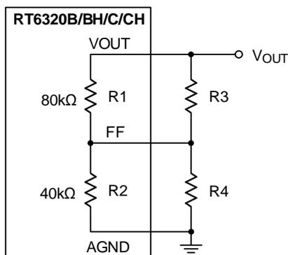
Figure 12. RT6320B/BH/C/CH Slightly Adjusts V<sub>OUT</sub> with FF Pin
