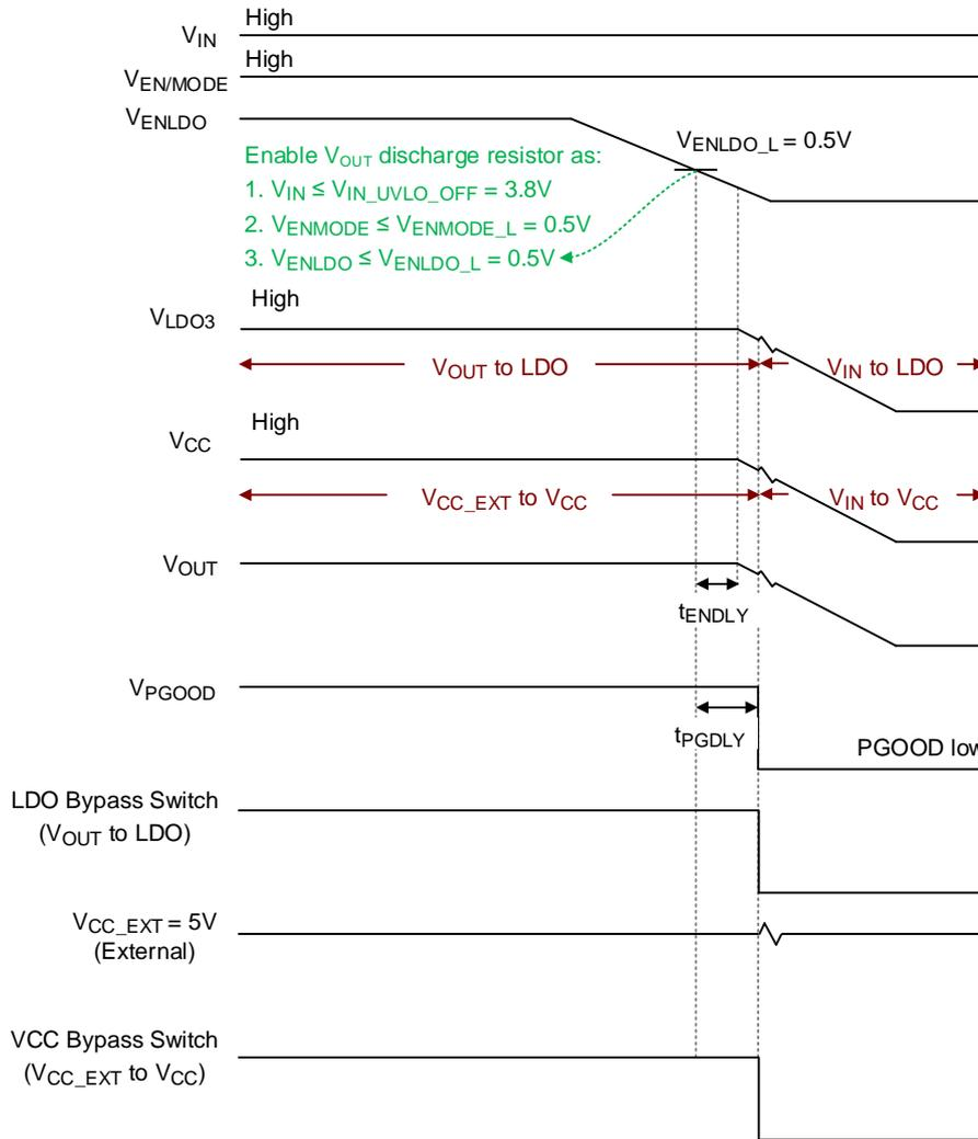
Figure 10. The RT6320B/BH ENLDO Pin Power Off
