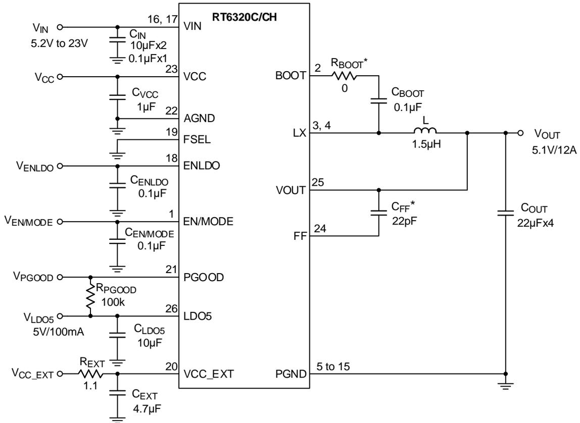
R<sub>BOOT</sub>\* : R<sub>BOOT</sub> is reserved for option. R<sub>BOOT</sub> must be less than 10Ω.
