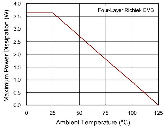
Figure 17. De-rating Curve of Maximum Power Dissipation
