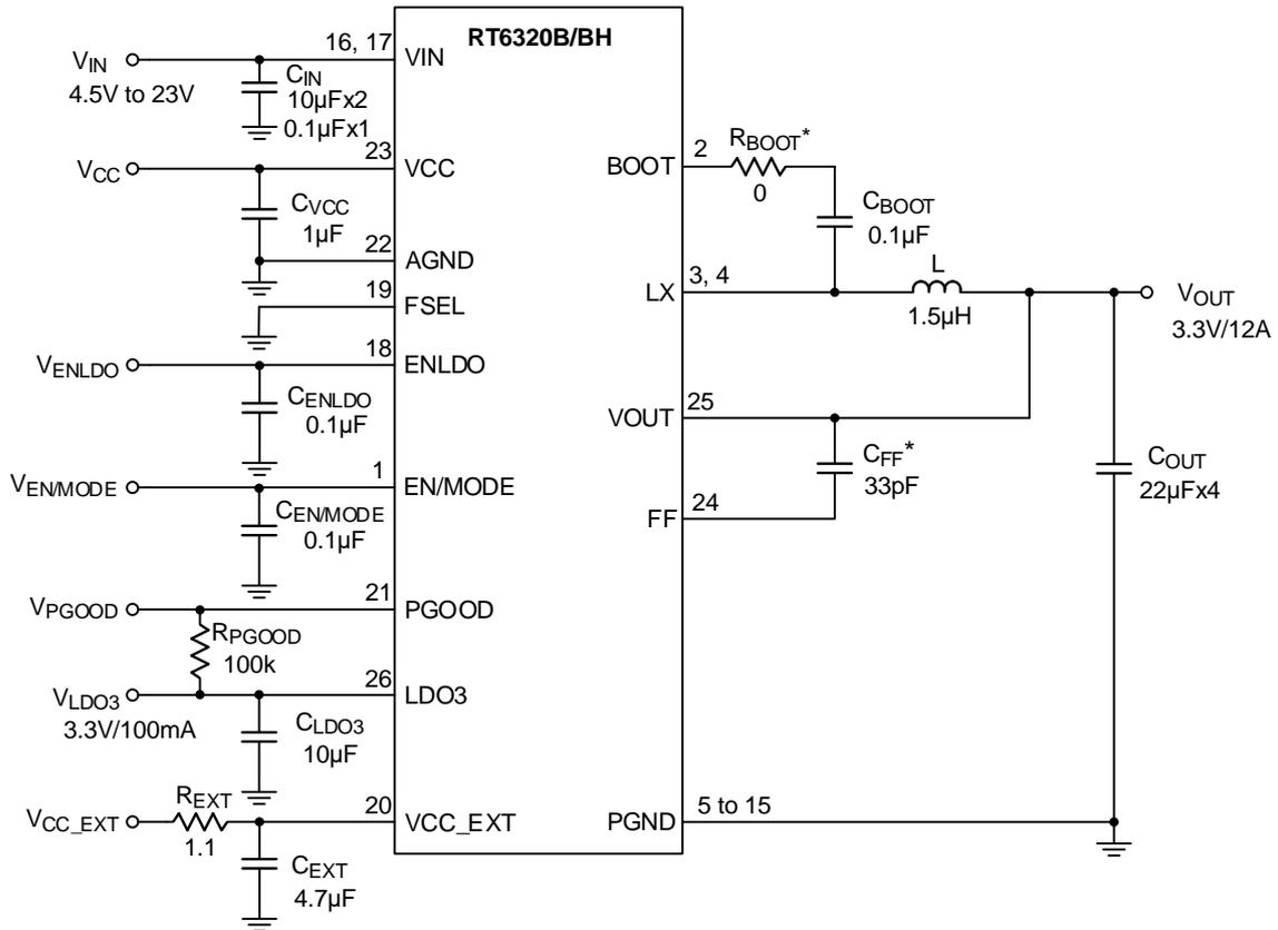
$R_{BOOT}^*$  :  $R_{BOOT}$  is reserved for option.  $R_{BOOT}$  must be less than  $10\Omega$ .
