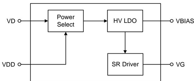
Figure 1. Power Selection Circuit
