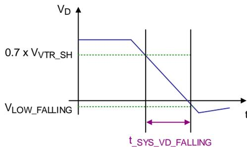
Figure 9. VD Falling Time Measurement Waveform
