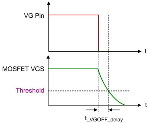
Figure 4. VG Turned Off Delay Time
