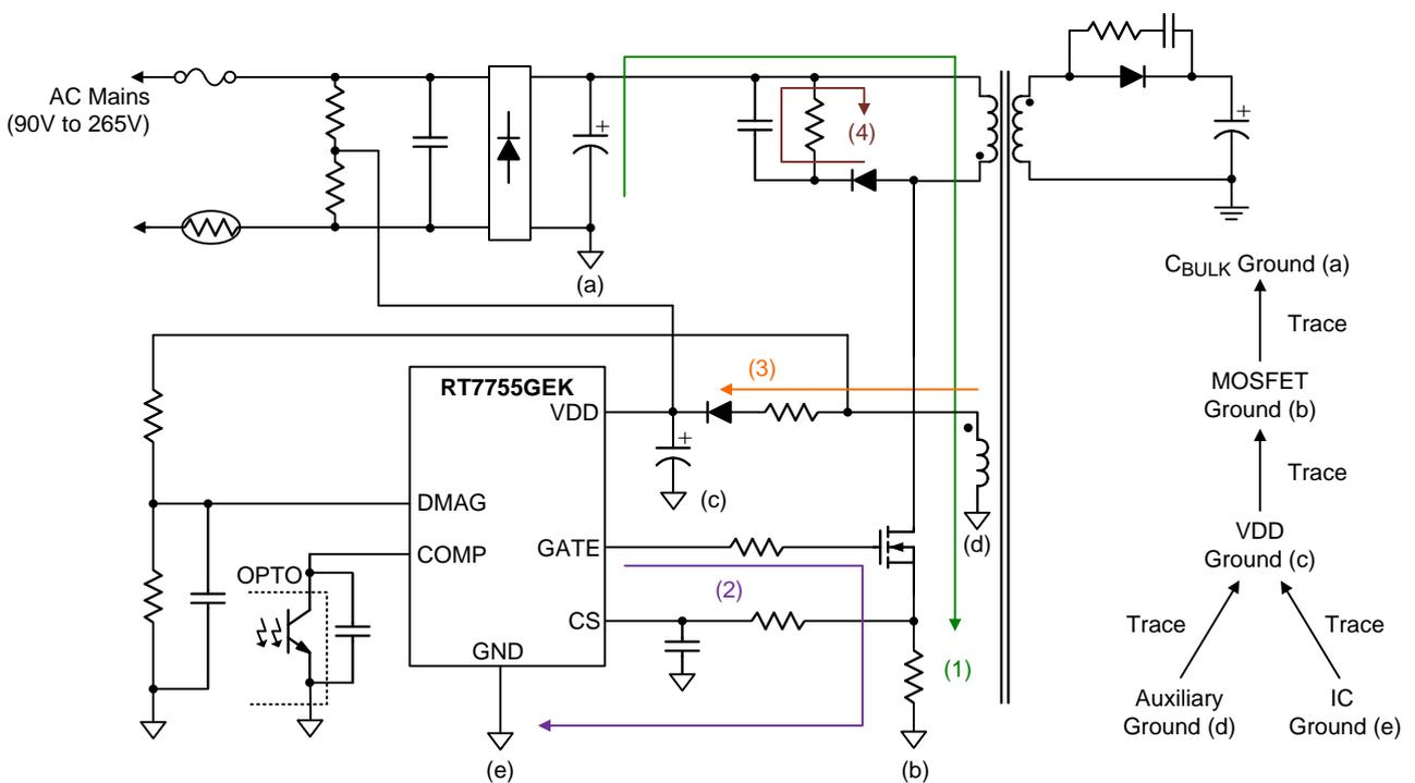
Figure 12. PCB Layout Guide
