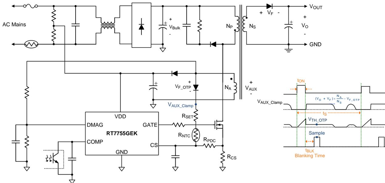
Figure 7. Application Circuit of External Over-Temperature Protection
