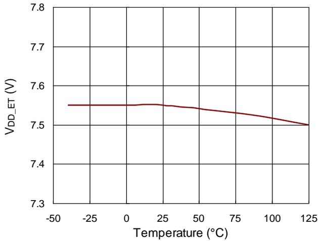
V<sub>DD\_ED</sub> vs. Temperature
