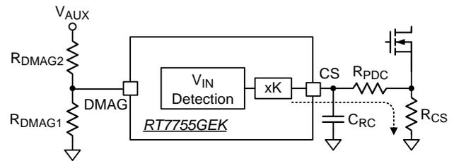
Figure 5. Functional Block Diagram of Line Compensation
