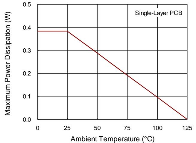
Figure 11. Derating Curve of Maximum Power Dissipation
