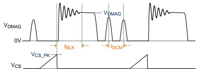
Figure 4. Resonant Oscillations on the DMAG Pin
