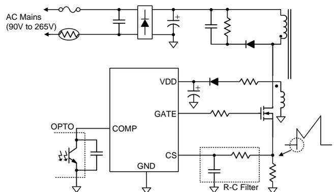
Figure 10. R-C Filter on the CS Pin
