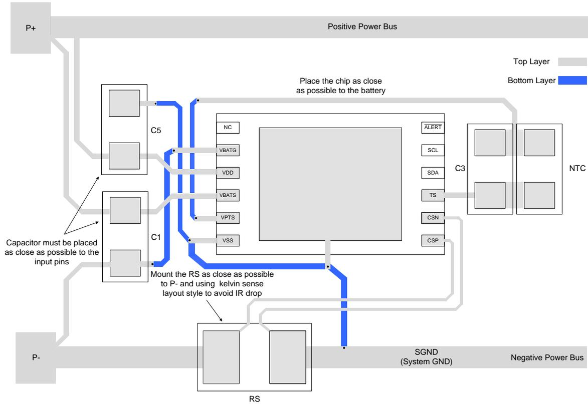
Figure 4. PCB Layout Guide for WDFN-12L 2.5x4 Package
