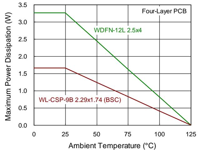
Figure 3. Derating Curve of Maximum Power Dissipation
