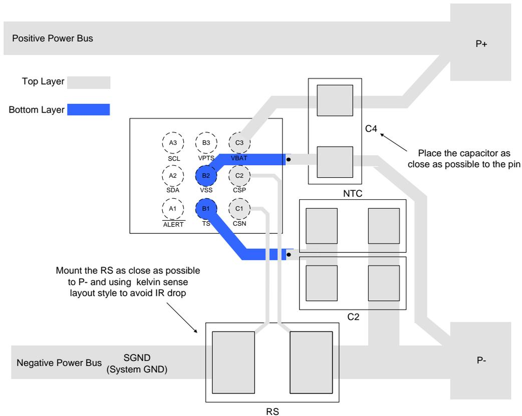
Figure 5. Low-Side Sensing PCB Layout Guide for WL-CSP-9B 2.29x1.74 (BSC) Package
