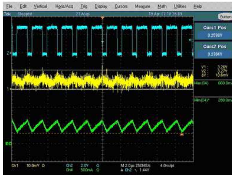
Figure 9. Ceramic 22µF 1210 (X5R) (Good)
