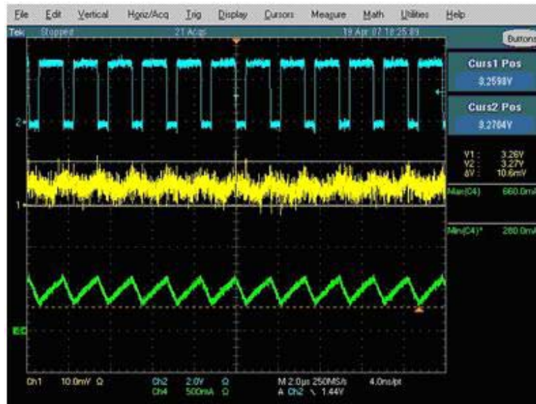
Figure 18. Ceramic 22 \mu F 1210(X5R) (Good)
