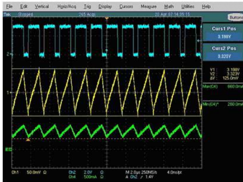
Figure 20. Electrolytic 100 \mu F (Ripple Too High)
