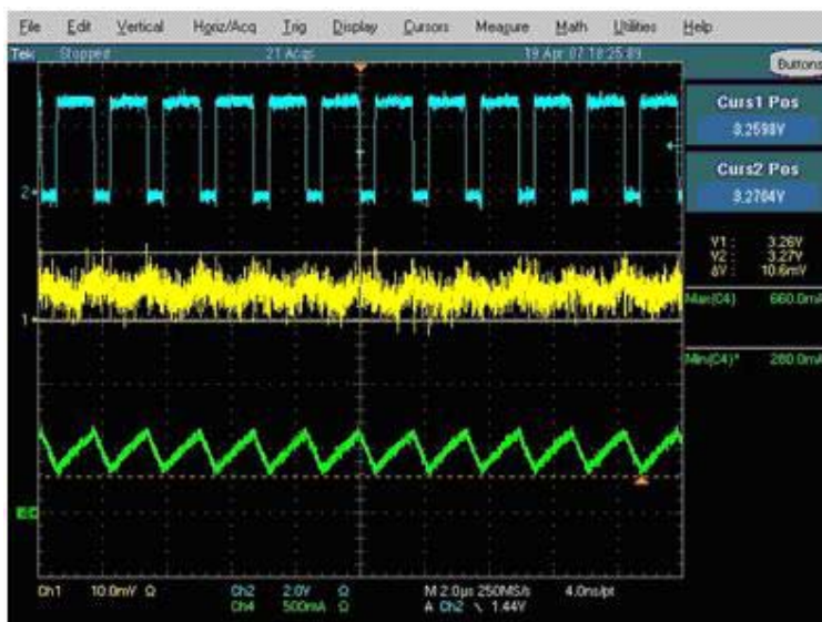
Figure 14. Ceramic 10 \mu F 0603 (X5R) (Good)
