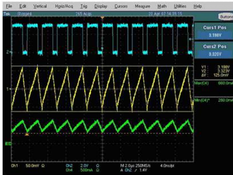
Figure 11. Electrolytic 100 \mu F (Ripple Too High)
