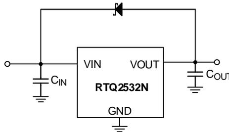
Figure 7. Application Circuit for Reverse Current Protection
