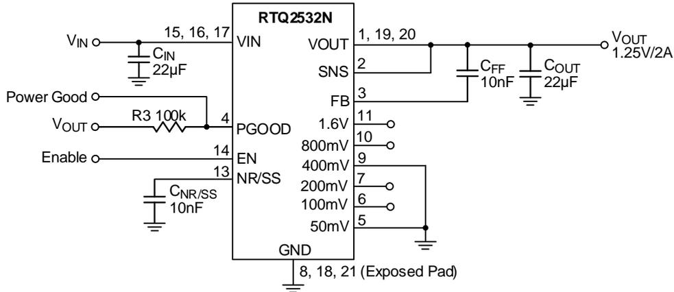
$$V_{OUT} = V_{REF} + 50mV + 400mV = 0.8V + 50mV + 400mV = 1.25V$$
