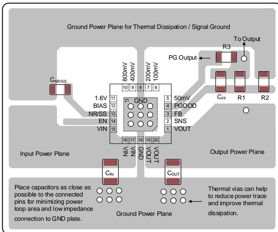
Figure 9. PCB Layout Guide
