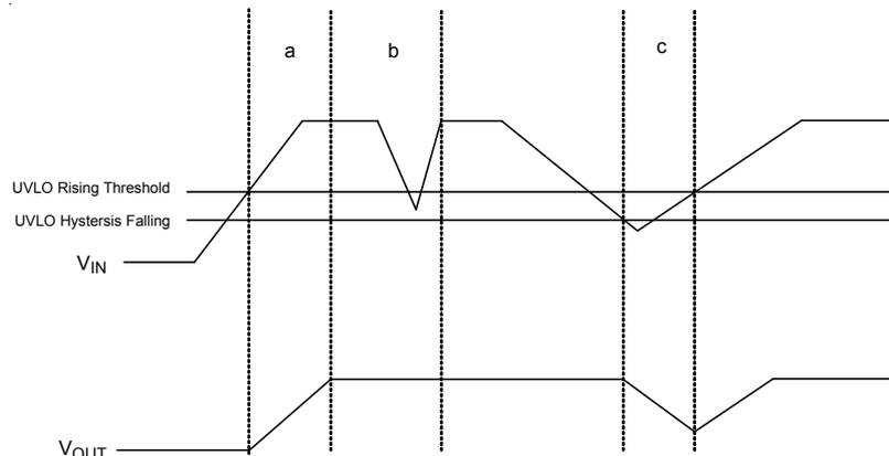
Figure 5. Under-Voltage Lockout Trapping Conditions and Output Variation
