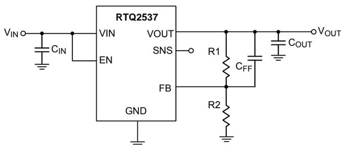
Figure 3. Output Voltage Set by External Resistors
