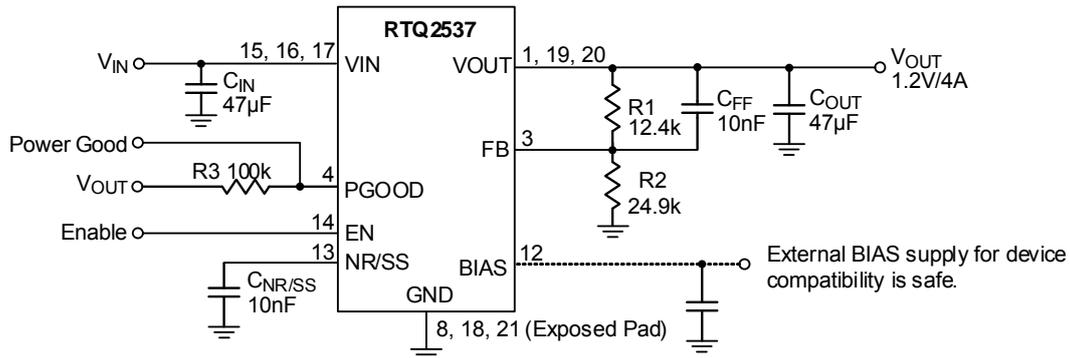
$$V_{OUT} = V_{REF} \times \left( 1 + \frac{R1}{R2} \right) = 0.8V \times \left( 1 + \frac{12.4k}{24.9k} \right) = 1.2V$$
