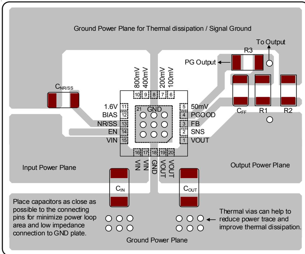
Figure 9. PCB Layout Guide
