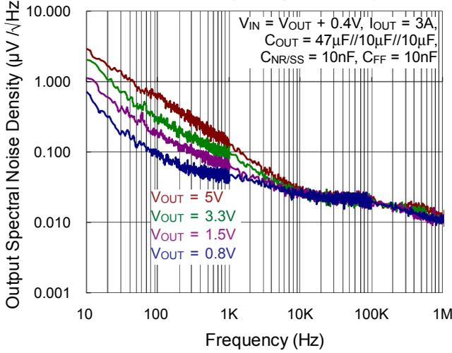
Output Noise vs. Frequency and Input Voltage
