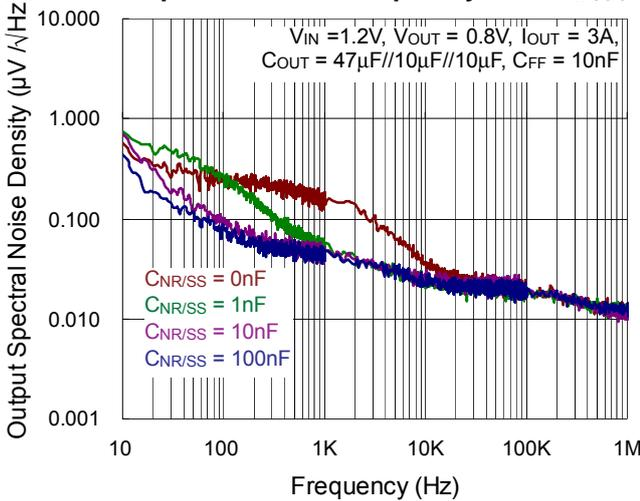
Output Noise vs. Frequency and CFF
