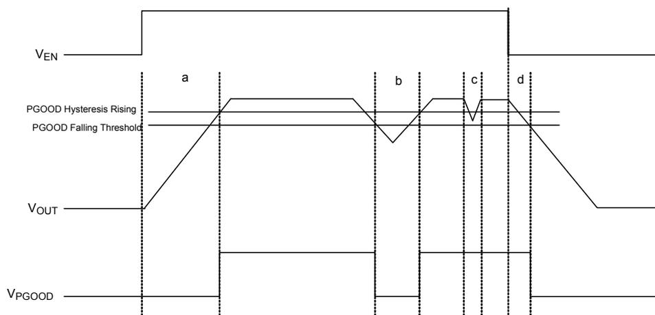
Figure 6. PGOOD Trigger Scenario with Different Operating Status
