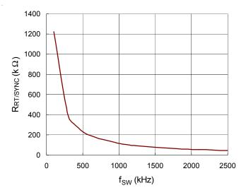
Figure 3. Switching Frequency vs. RRT/SYNC
