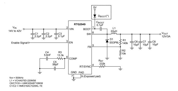
\*: While the input voltage is below 5.5V or duty ratio is higher than 65%, an external bootstrap diode must be added between an external 5V voltage supply and the BOOT pin to enhance the drive capability for the high-side MOSFET. Refer to the Application Information for more details on the external bootstrap diode design.
