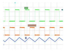
Figure 14. Synchronization Mode in CCM
