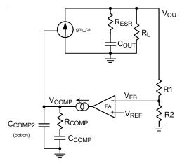
Figure 8. Simplified Equivalent Circuit of Buck with PCMC
