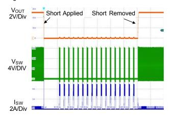
Figure 2. Short-Circuit Protection and Recovery
