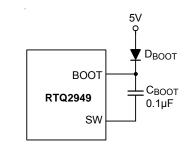
Figure 9. External Bootstrap Diode
