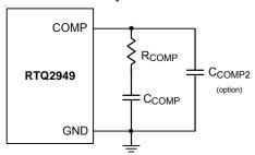
Figure 7. External Compensation Components
