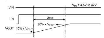
Figure 1 Start-Up Sequence for RTQ2949GQW
