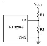
Figure 6. Output Voltage Setting
