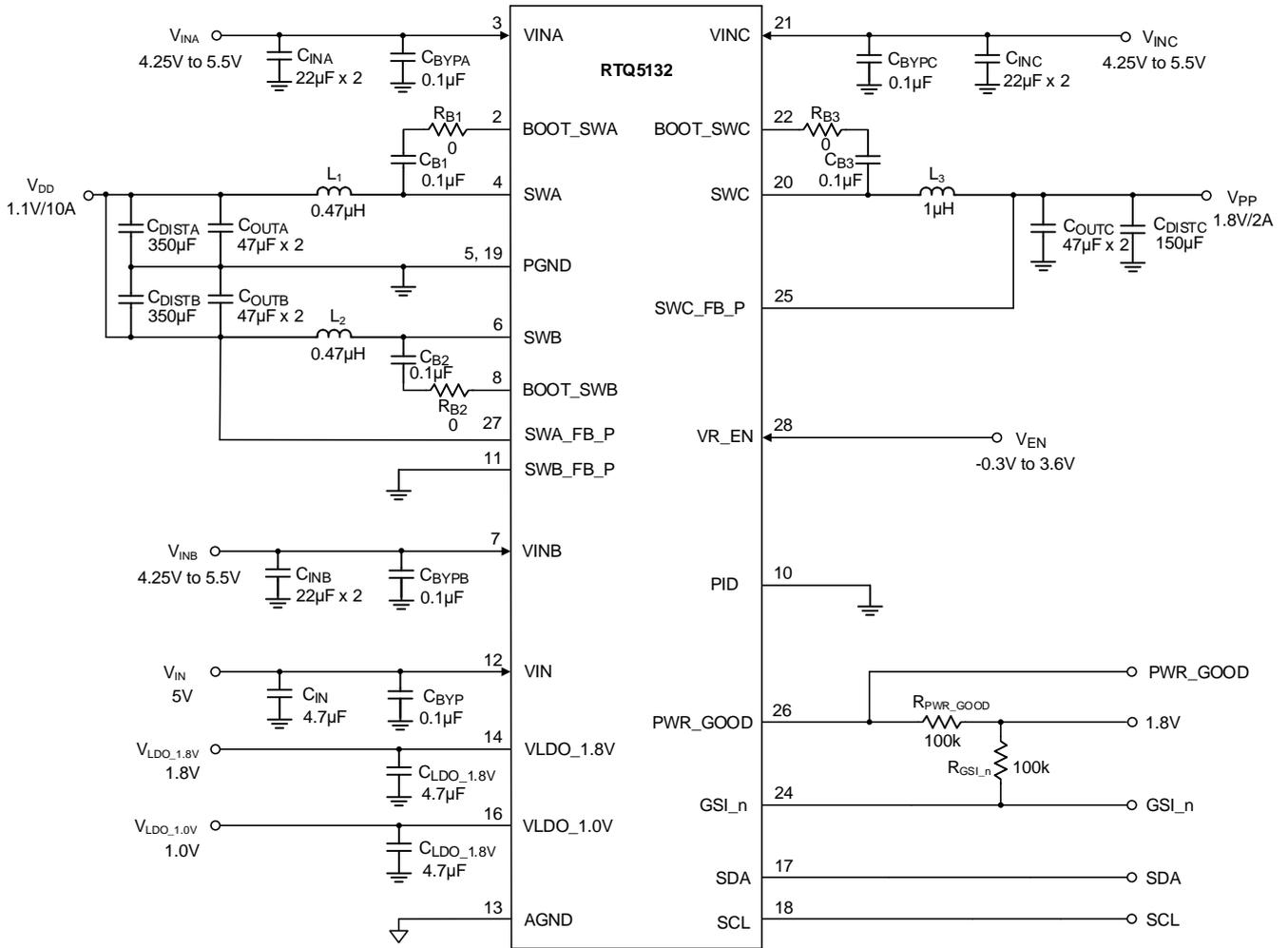
Figure 13. Typical Application Circuit when SWA and SWB are combined as Two Phase, Single Output Rail.
