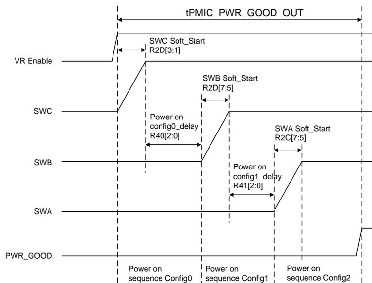
Figure 7. RTQ5132 Rails Power On Timing
