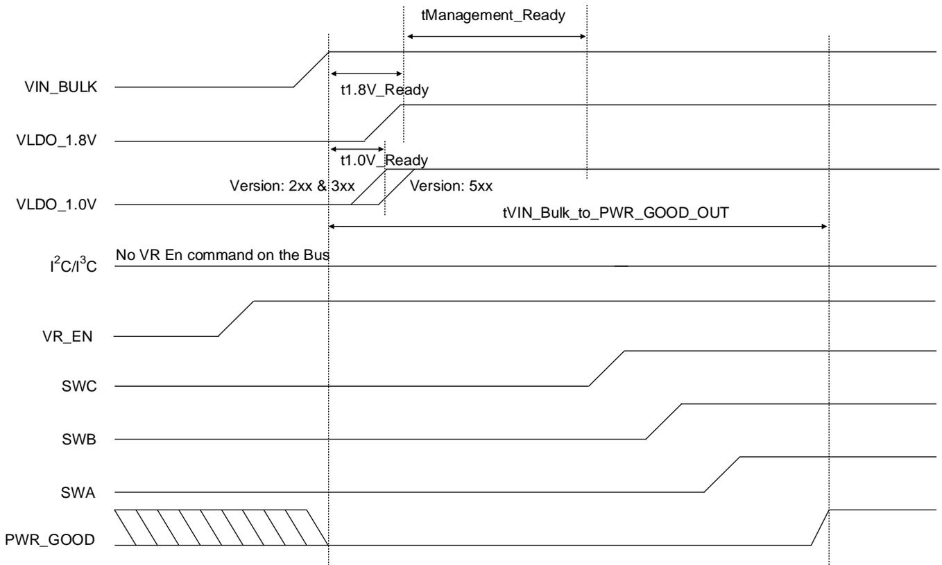
Figure 4. Power Up Sequence; VR\_EN pin High before VIN\_Bulk Ramp; No Bus Command
