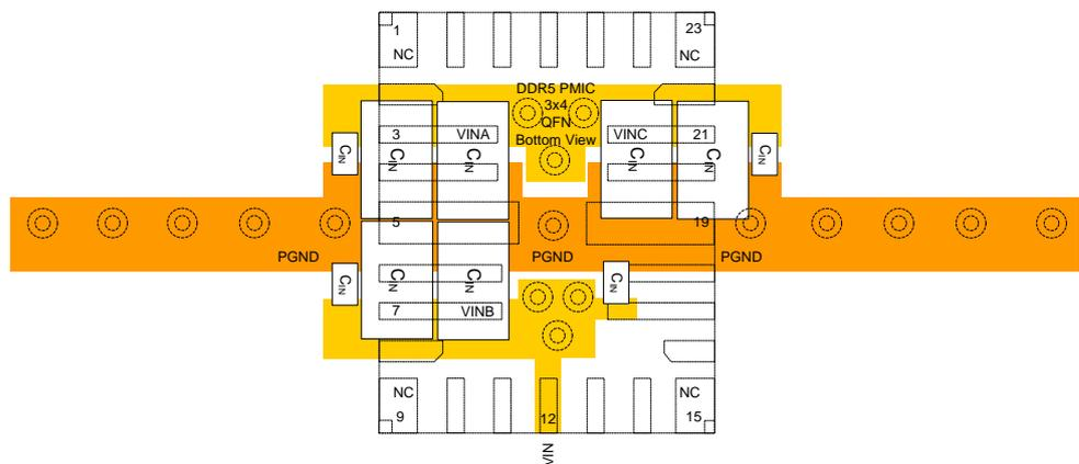
Figure 22. RTQ5132 Layout Guide (Bottom Layer)
