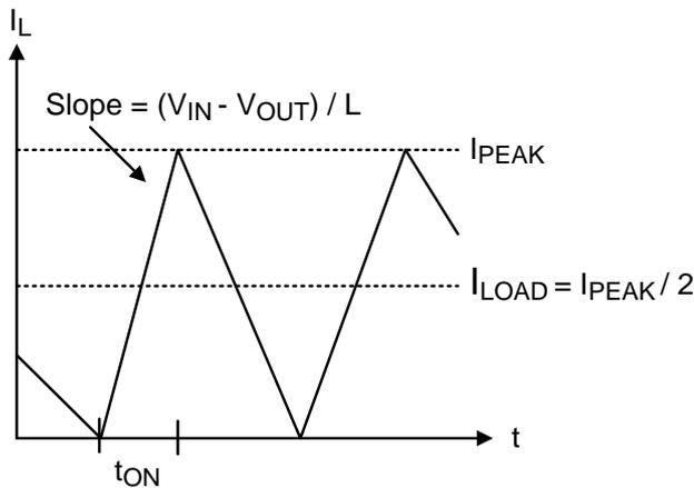
Figure 12. Boundary Condition of DEM/CCM
