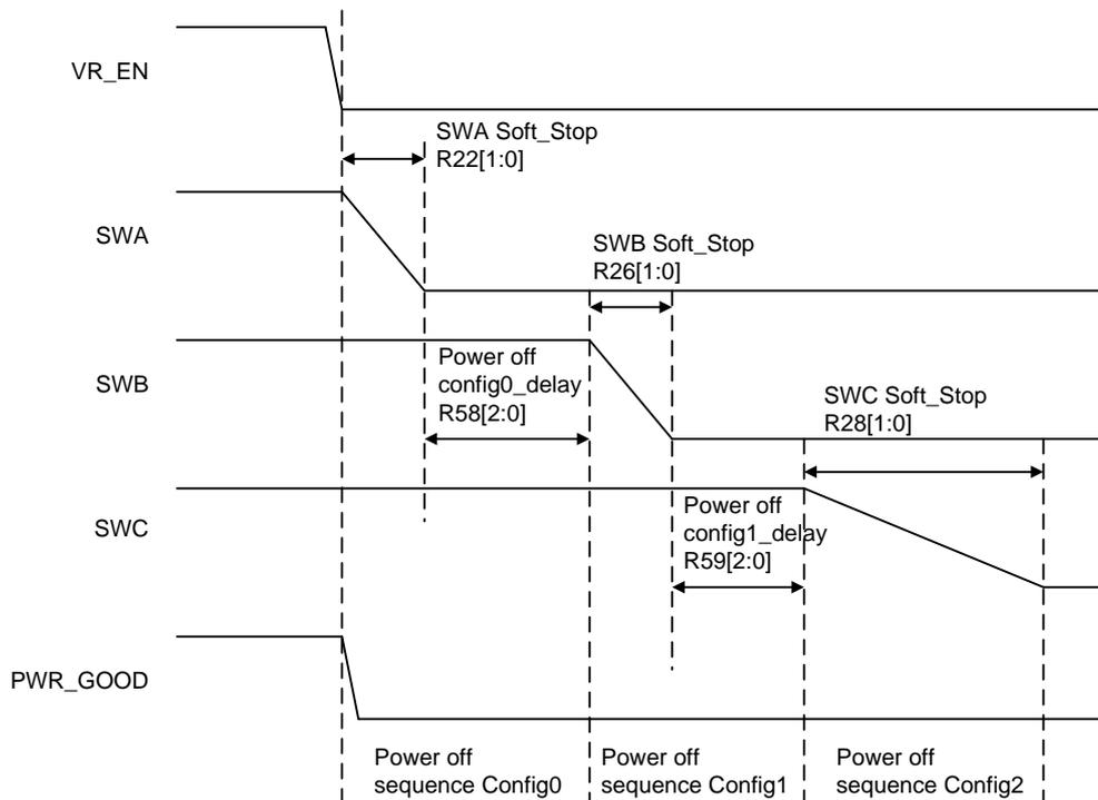
Figure 8. PMIC Power Off Timing Due to Internal Fault Condition
