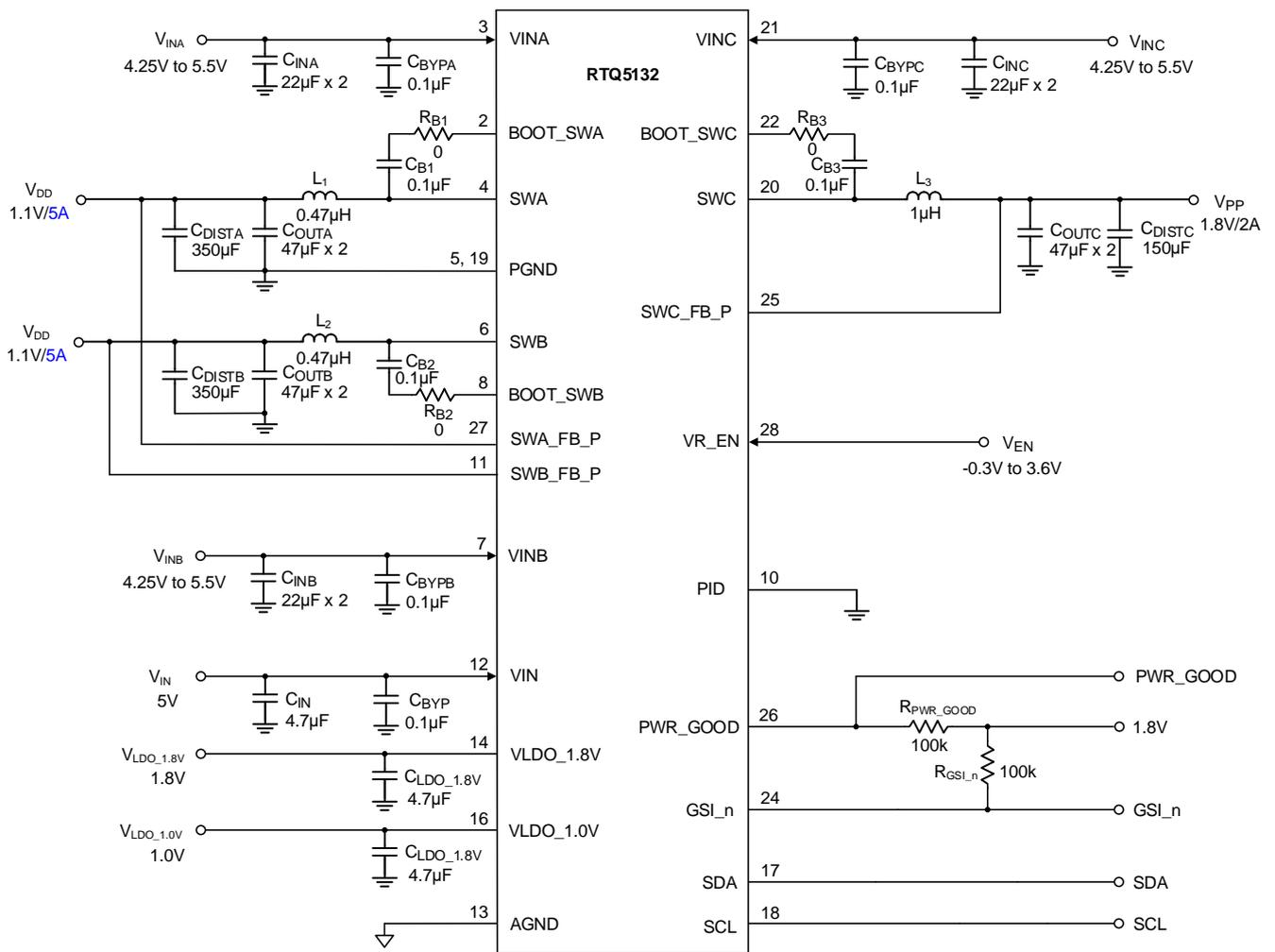
Figure 14. Typical Application Circuit when SWA and SWB are separated for 2-Outputs.
