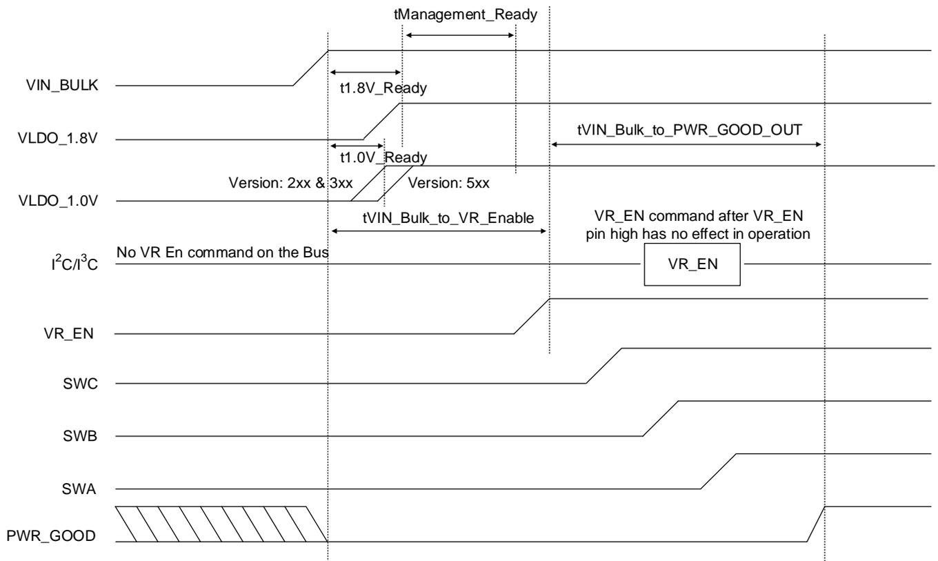
Figure 6. PMIC Power Up Sequence; w/ VR\_EN Pin followed by Bus Command
