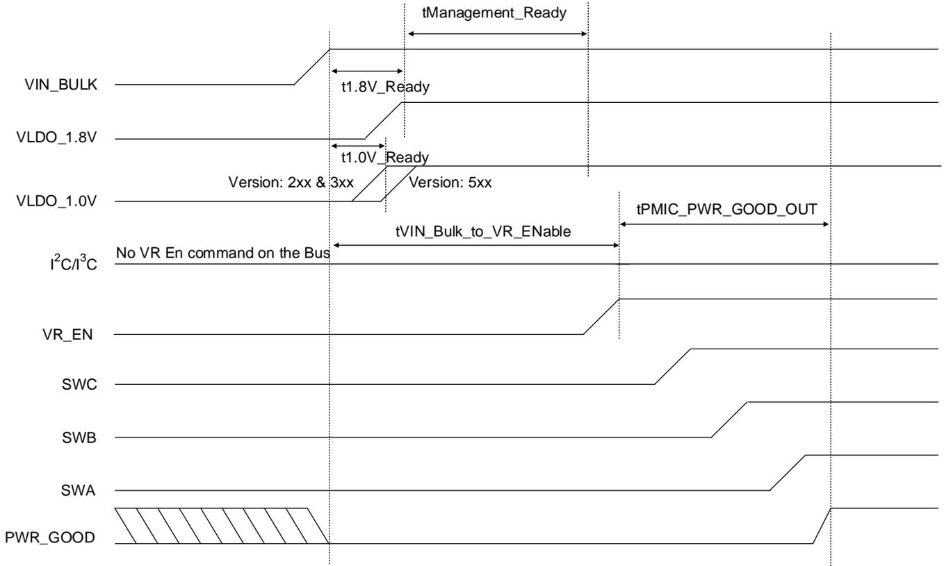
Figure 3. Power Up Sequence; VR\_EN pin High after VIN\_Bulk Ramp; No Bus Command
