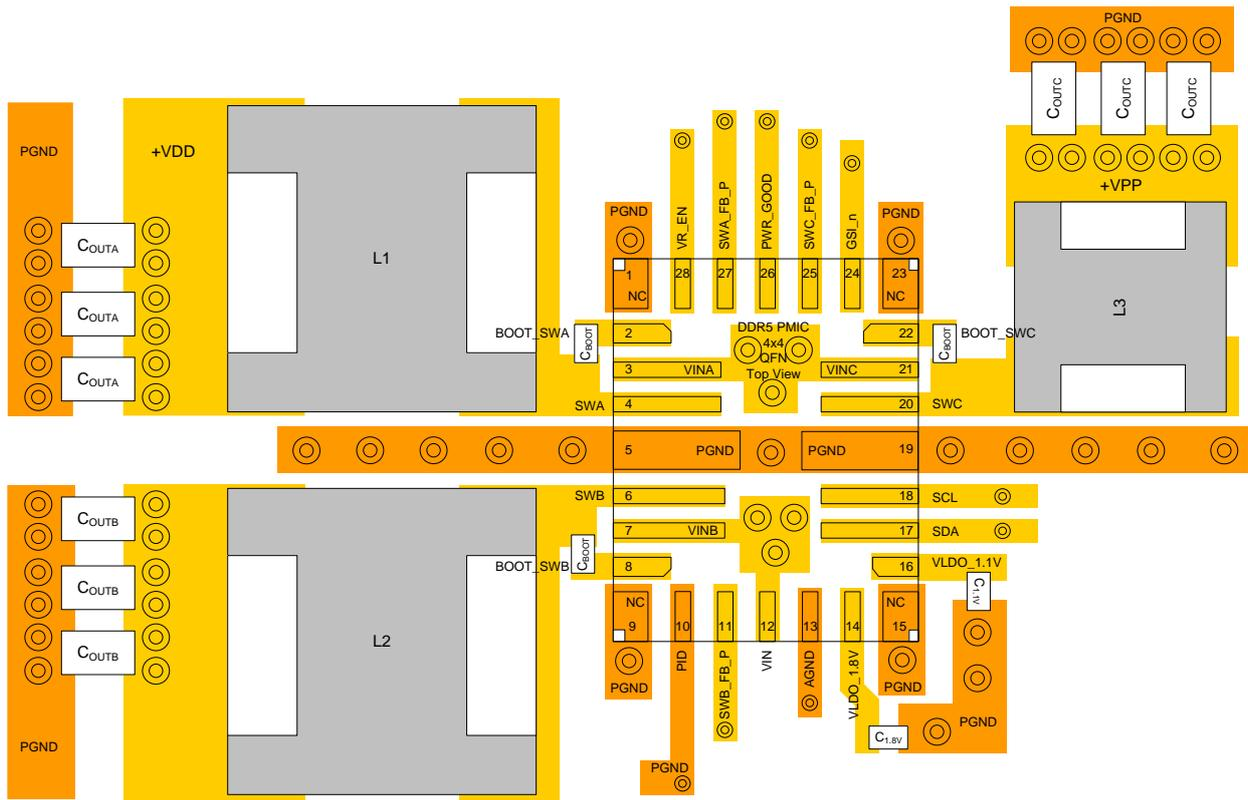
Figure 21. RTQ5132 Layout Guide (Top Layer)
