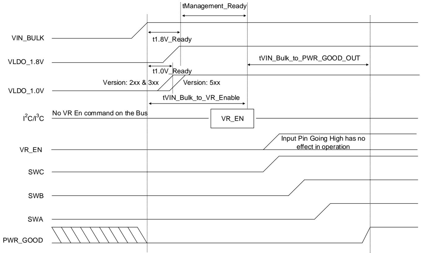
Figure 5. PMIC Power Up Sequence; w/ VR\_EN Pin followed by Bus Command
