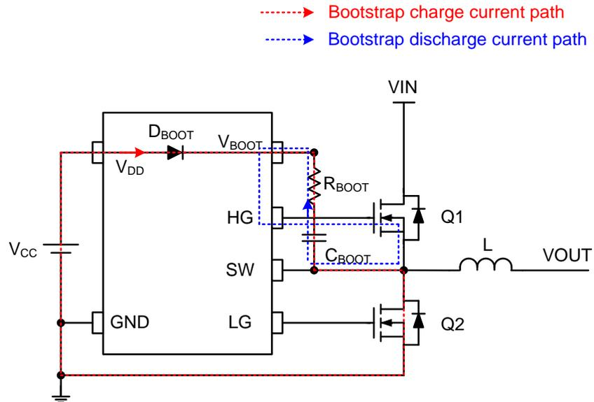
Figure 19. Bootstrap Power Supply Circuit
