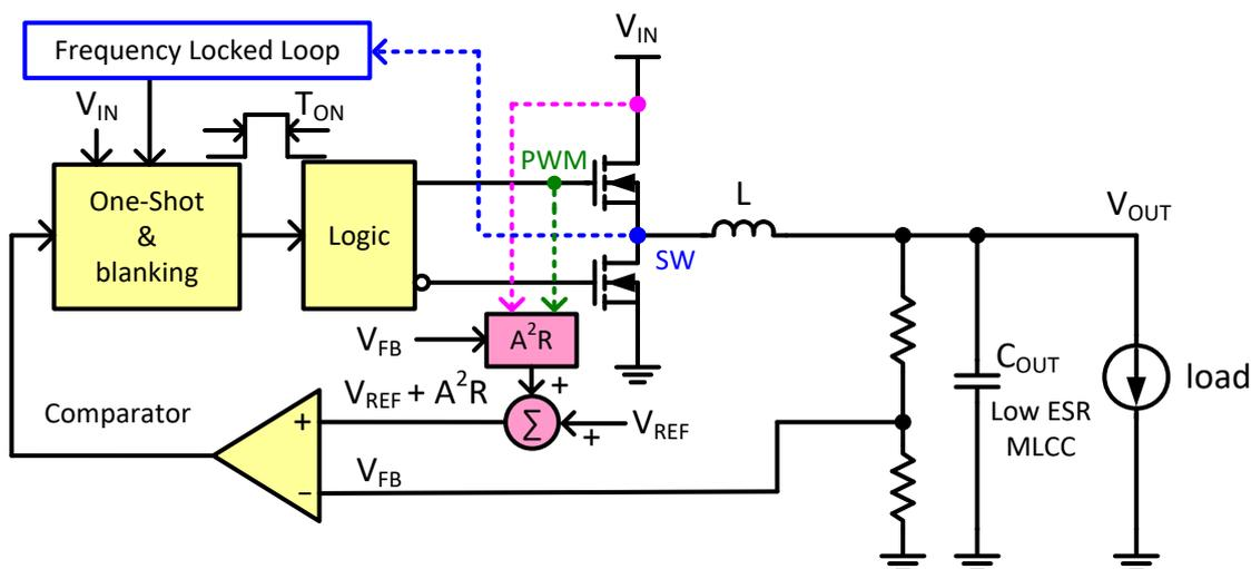
Figure 10. A<sup>2</sup>RCOT Control Mechanism
