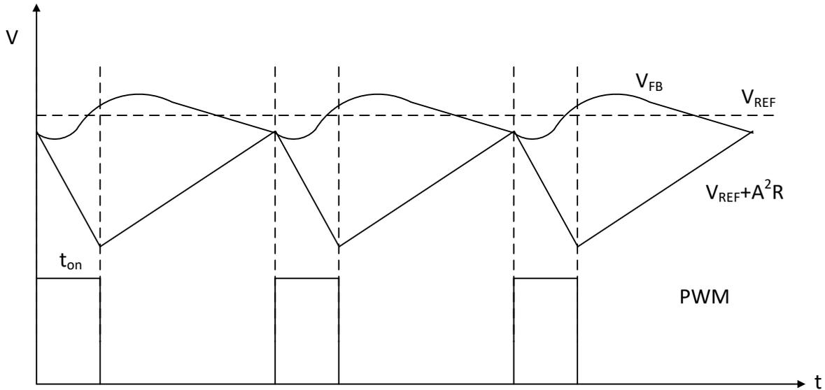
Figure 11. A²RCOT PWM Control Diagram
