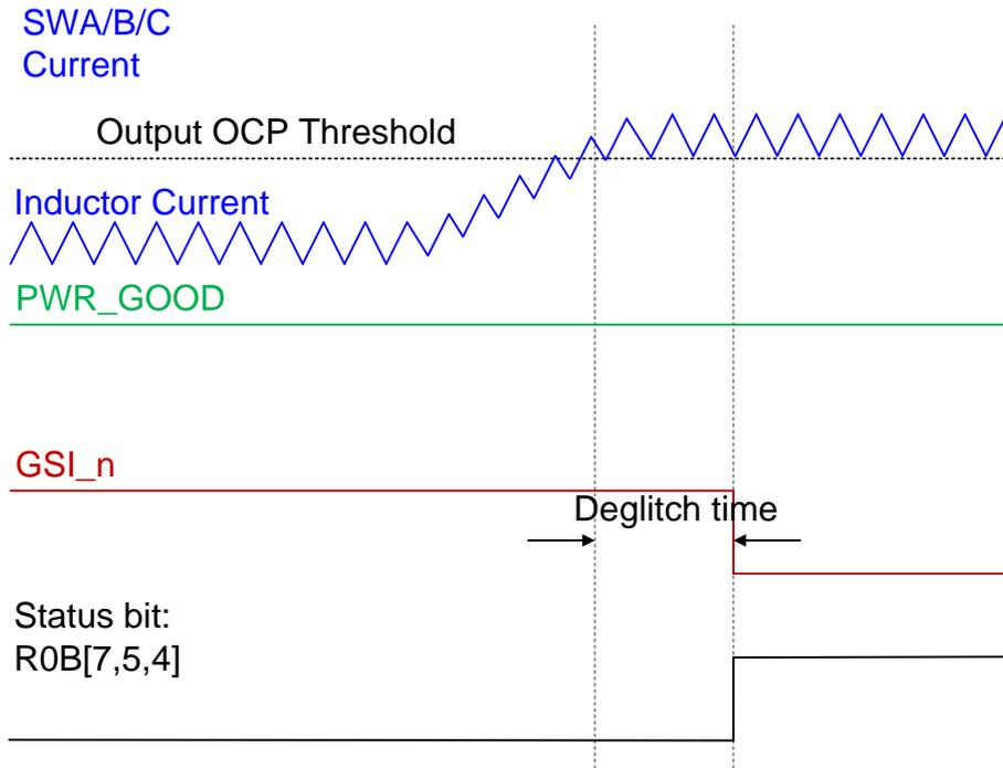
Figure 9. Output Current Limiter Protection
