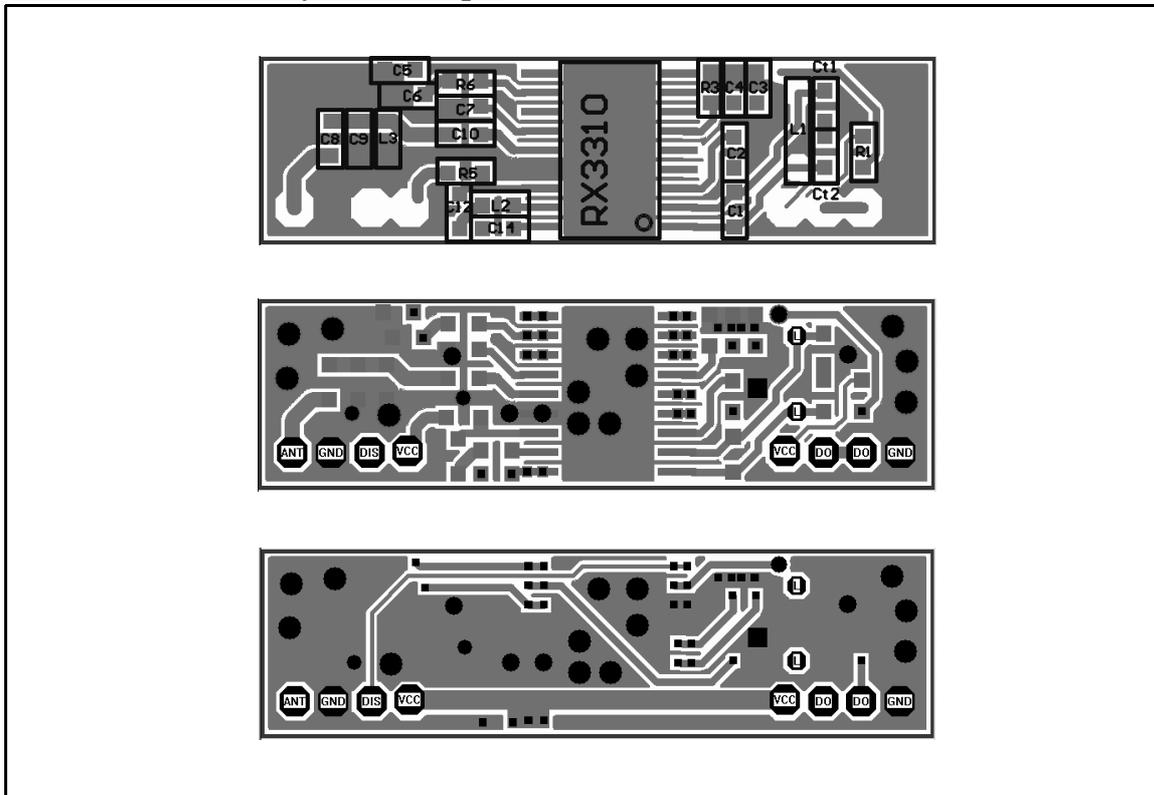
From top to bottom: Component side of printed-circuit board, top side, bottom side.
