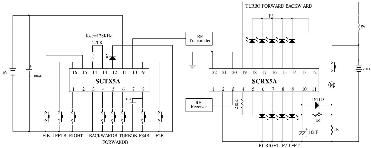
SCTX5A output pin (so) has an inverted phase with SCR5A input ( SI ). If SCTX5A&SCR5A are connected without using a RF module. An inverter has to be inserted between this 2 pins.
