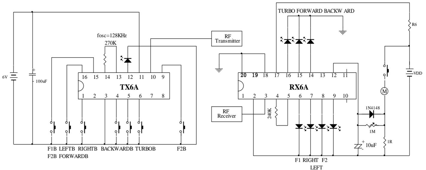
SCTX6A output pin (so) has an inverted phase with SCRX6A input (SI). If SCTX6A&SCRX6A are connected without using a RF module. An inverter has to be inserted between this 2 pins.
