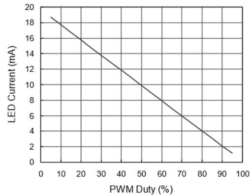
The LED current can be calculated by the following Equation:
