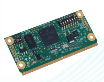
The RainboW-G16M-µMXM SOM is based on Freescale's Vybrid VF6xx/VF5xx family solution combining ARM Cortex-A5 and Cortex-M4 cores, which often eliminate the need for an external MCU for real time control applications. Vybrid devices also provide a powerful combination of on-chip encryption; secure boot, anti-tamper and anti-clone capabilities to secure sensitive or critical infrastructure applications such as smart grid or industrial control.
