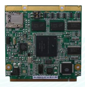
iWave Systems launched its latest low power, high performance, Qseven compatible SOM module based on Freescale's i.MX515 ARM Cortex-A8 Application processor. This module offers high performance processing with a high degree of functional integration, aimed at the growing Industrial automation, healthcare and general embedded control applications. The board supports the major operating systems including Linux, WinCE6.0, Android 2.3 and QNX.
