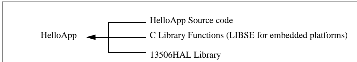
Figure 14-1: Components needed to build 13506 HAL application
